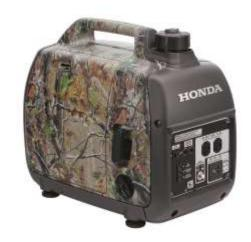
features a totally enclosed body that results in noticeably quieter performance to enhance the outdoor experience. Its two-tiered noise dampening system reduces noise to 59 decibels (db) at rated load and 53 db (quieter than normal speech) at one-quarter load. What's more, this 2000-watt model can simultaneously power a computer, TV, coffee pot, and portable refrigerator.
