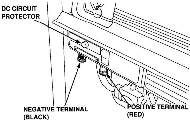
4. Connect the negative (-) battery cable to the battery negative (-) terminal.
