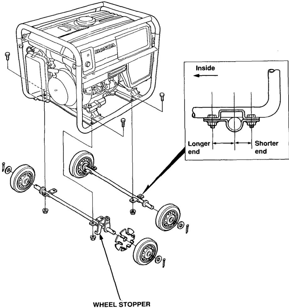
**NOTE:** Install the shaft with wheel stopper facing engine side.
