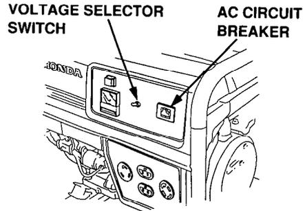
Do not exceed the current limit specified for any one receptacle. If an overloaded circuit causes the AC circuit breaker or circuit protector to switch OFF, reduce the electrical load on the circuit, wait a few minutes and then reset the circuit breaker.
