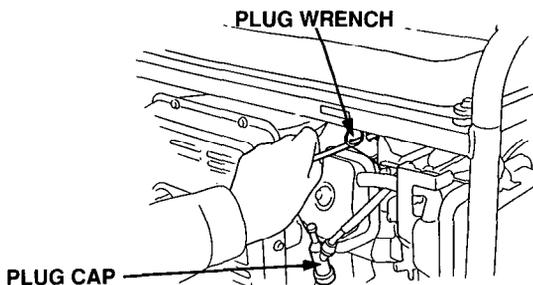
5. Visually inspect the spark plug. Discard it if the insulator is cracked or chipped. Clean the spark plug with a wire brush if it is to be reused.
