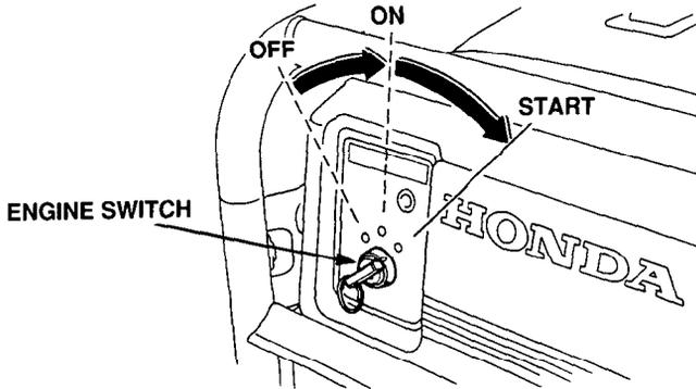
Return the key to the ON position once the engine has started. Do not use the starter for more than 5 seconds at a time. If the engine fails to start, release the switch and wait 10 seconds before operating the starter again.
