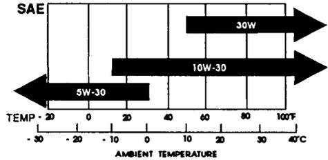
SAE 10W-30 is recommended for general, all-temperature use. Other viscosities shown in the chart may be used when the average temperature in your area is within the indicated range.
