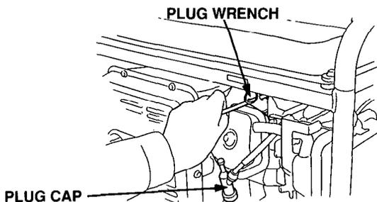
5. Visually inspect the spark plug. Discard it if the insulator is cracked or chipped. Clean the spark plug with a wire brush if it is to be reused.
