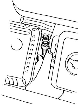
7. After a new spark plug has been seated by hand, it should be tightened  $1/2$  turn with a wrench to compress its washer.
