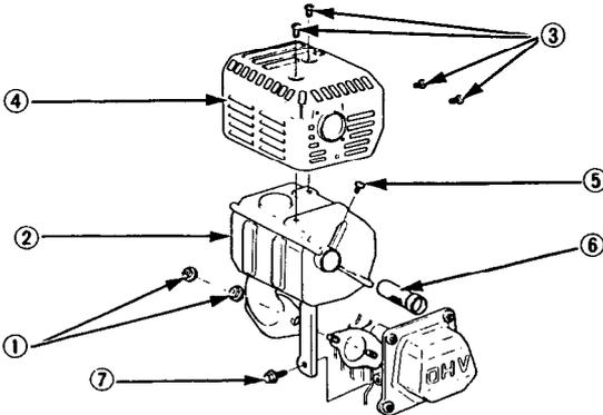
4. Check for carbon deposits around the exhaust port and the spark arrester. Carefully clean the spark arrester with a brush as shown.
