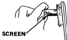
NOTE: The spark arrester must be free of breaks and holes. Replace, if necessary.
