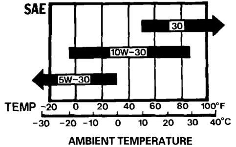
SAE 10W-30 is recommended for general, all-temperature use. Other viscosities shown in the chart may be used when the average temperature in your area is within the indicated range.
