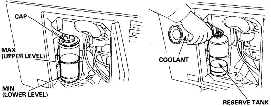
The engine protection system will automatically stop the engine if the coolant gets too hot, which may occur if the coolant level is too low. To avoid the inconvenience of an unexpected shutdown, inspect the coolant level in the reserve tank regularly.
