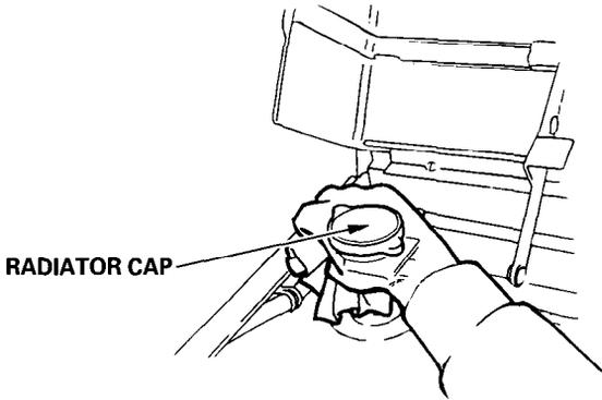
2. Fill the radiator with coolant, and reinstall the radiator cap. Tighten the cap securely.
