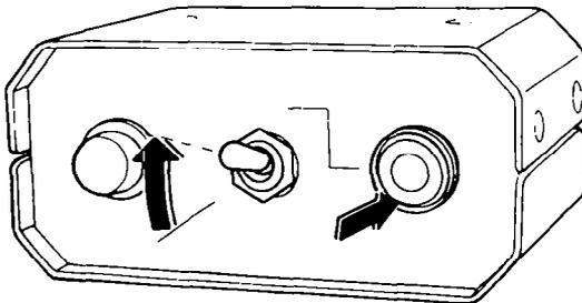
6. Depress the starter button until the pilot lamp is on.
