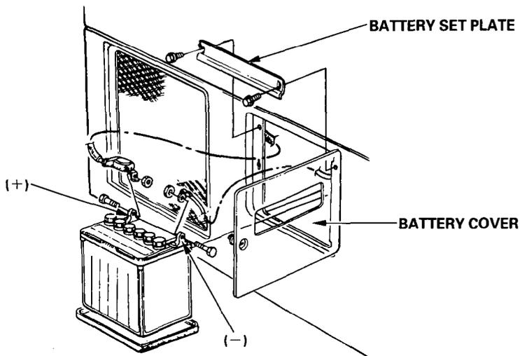
4. Remove the battery from the battery tray.
