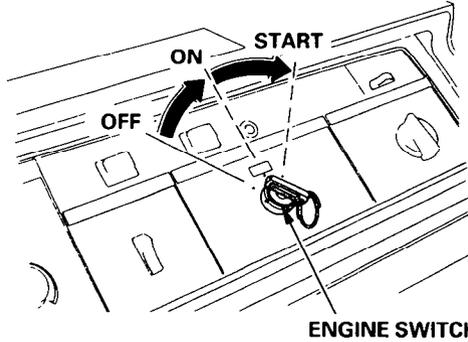
Return the key to the ON position once the engine has started. Do not use the starter for more than 5 seconds at a time. If the engine fails to start, release the switch and wait 10 seconds before operating the starter again.
