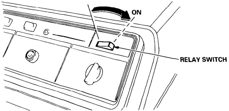
5. Flip the remote control engine switch up to ON.
