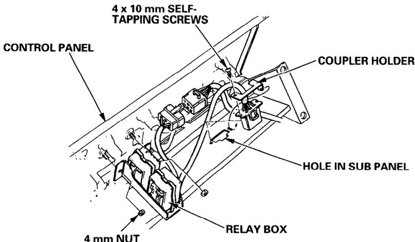
3. Remove the 6-P coupler with a jumper wire from the wire harness female coupler. Connect the relay box 6-P male coupler to the wire harness female coupler.
