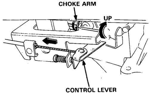
2. If adjustment is necessary, loosen the control cable lock nuts, and move the adjuster up or down as required. Tighten the lock nuts, and recheck the carburetor choke arm position.
