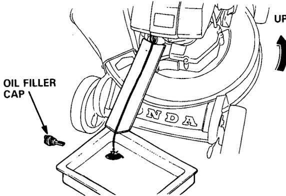
3. Refill to the "Upper" level mark with the recommended oil (see p.12). Tighten the cap securely to prevent leakage.
