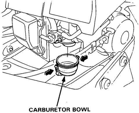
C. Reinstall the bowl, connect the fuel tube and turn the fuel valve off.
