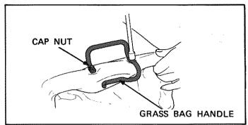
6. Expose the two stud bolts through the holes in the bag and install the grass bag handle to the bag with two 6 mm cap nuts.
