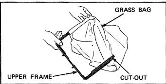
1. Work the upper frame into the grass bag with the 2. Place the anti-sag rod in the bag and secure it to the cut-out ends forward.
