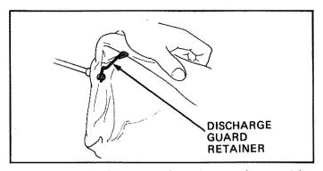
5. Install the discharge guard retainer as shown with a 6 mm bolt, nut and washer.
