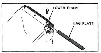
4. Work the bag plate into the grass bag and tighten them to the lower frame with three 6 mm bolts.
