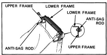
3. Point the lipped edge of the lower frame forward, place the bends into the cut-outs in the upper frame and tighten the lower frame to the upper frame together with the anti-sag rods using two 6 mm 12 flanged bolts.
