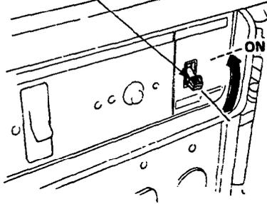
4. Turn the engine switch on.
