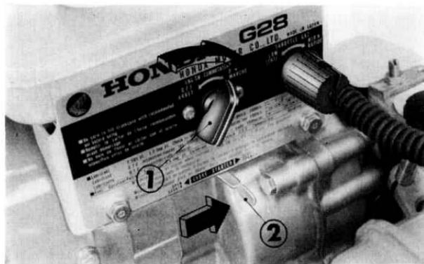
① Engine switch (fuel cock) ② Choke lever
