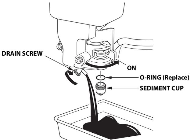
3. After all the fuel has drained into the container, tighten the drain screw securely.
