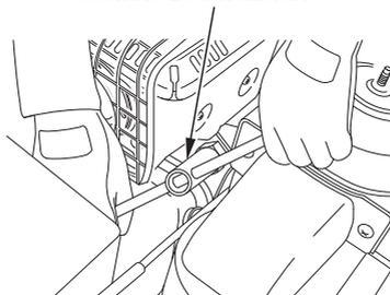
4. Inspect the spark plug. Replace it if the electrodes are worn, or if the insulator is cracked or chipped.
