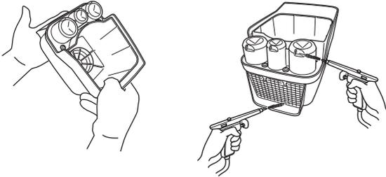
7. Wipe dirt from the inside of the air cleaner case and cover using a moist rag. Be careful to prevent dirt from entering the air duct that leads to the carburetor.
