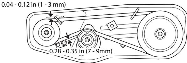
8. After adjustment has been completed, fasten the belt stopper bolts and engine mounting bolts securely.
