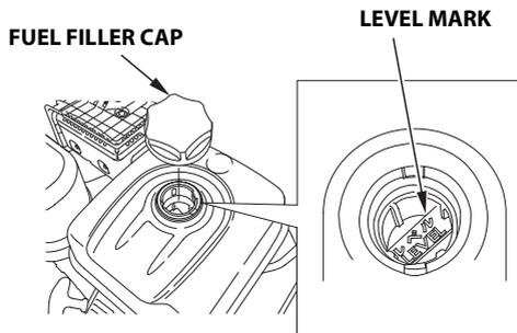
Refuel in a well-ventilated area before starting the engine. If the engine has been running, allow it to cool. Refuel carefully to avoid spilling fuel. Do not fill the fuel tank above the fuel level mark. After refueling, tighten the fuel tank cap securely.
