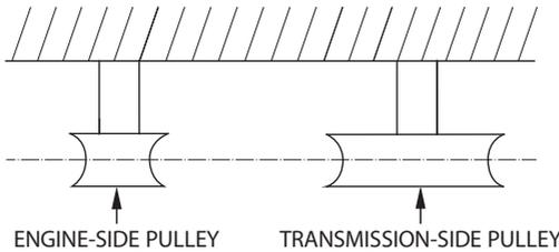
7. Squeeze the clutch lever, and adjust the clearance between the belt stoppers, as illustrated.
