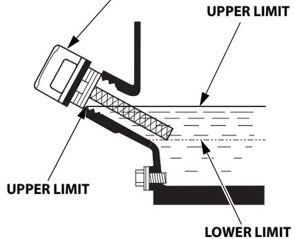
3. If the oil level is low, fill to the edge of the oil filler hole with the recommended oil (see page 34).
