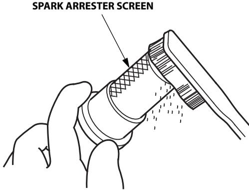
4. Install the spark arrester and the muffler protector in the reverse order of disassembly.
