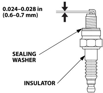
If reinstalling the used spark plug, tighten 1/8–1/4 turn after the spark plug seats.
