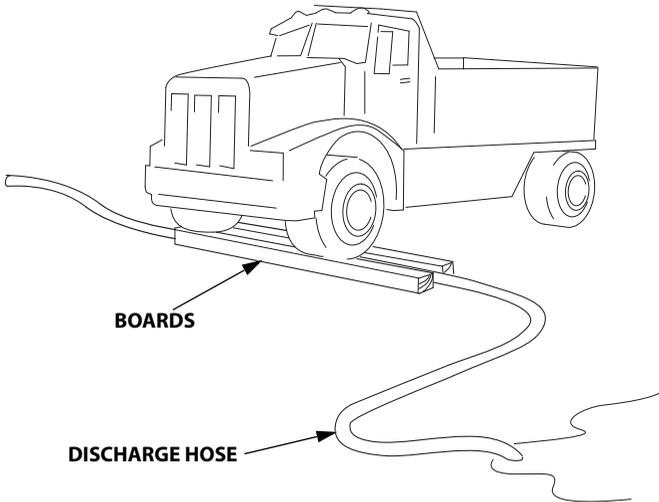
Driving over a discharge hose while the pump is running, or even possibly when the pump is stopped, may cause pump case failure.
