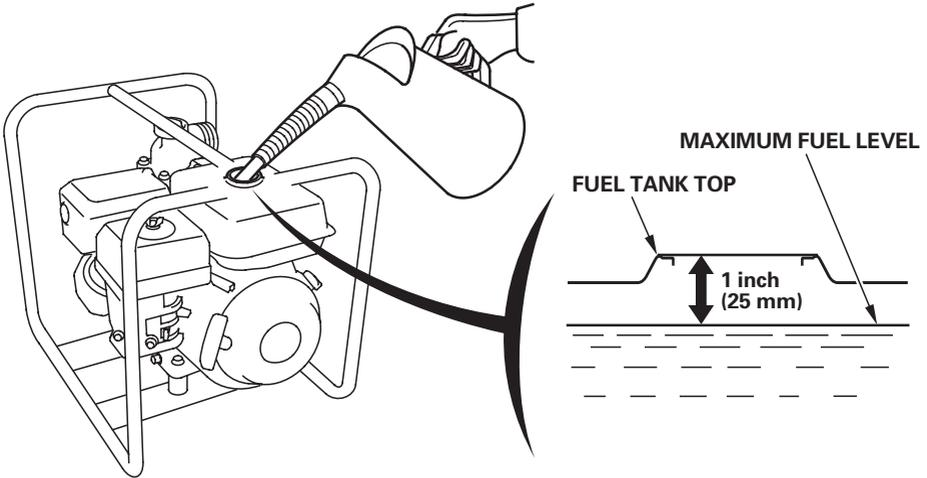
Refuel in a well-ventilated area before starting the engine. If the engine has been running, allow it to cool. Refuel carefully to avoid spilling fuel. Do not fill the fuel tank completely. Fill tank to approximately 1 inch (25 mm) below the top of the fuel tank to allow for fuel expansion. It may be necessary to lower the fuel level depending on operating conditions.
