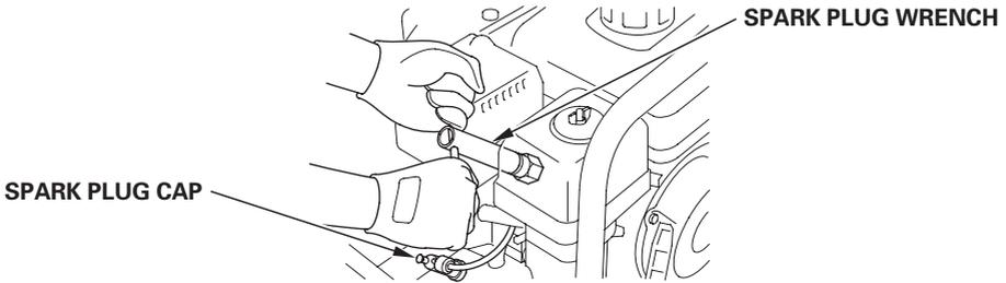
3. Inspect the spark plug. Replace it if the electrodes are worn, or if the insulator is cracked or chipped.
