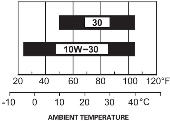
SAE 10W-30 is recommended for general use. Other viscosities shown in the chart may be used when the average temperature in your area is within the recommended range.
