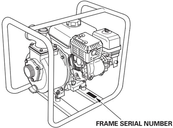
Record the frame serial number (if assigned) and the engine serial number in the space below. You will need these serial numbers when ordering parts, and when making technical or warranty inquiries (see page 59).
