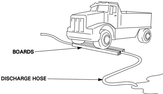
Driving over a discharge hose while the pump is running, or even possibly when the pump is stopped, may cause pump case failure.
