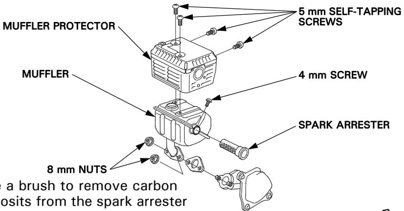
4. Use a brush to remove carbon deposits from the spark arrester screen. Be careful to avoid damaging the screen.
