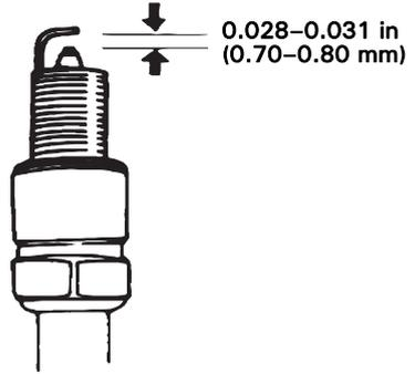
5. Install the spark plug carefully, by hand, to avoid cross-threading.
