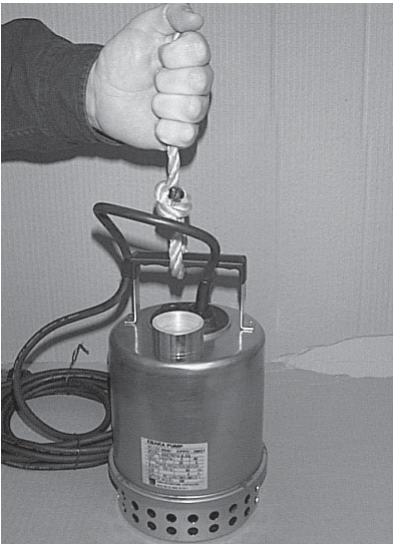
Rope attached to the manual pump for lifting and installation.
