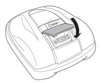
When the lawn mower is docked at the docking station, press the manual STOP button.
