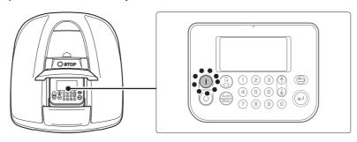
The power turns on, and the initial setup screen on the control panel is displayed.
