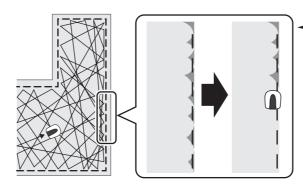
If the edge cutting setting is enabled, the lawn mower goes around your lawn along the boundary wire to mow the edge before starting the usual mowing.
