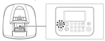
The power turns on, and the startup screen on the control panel is displayed.
