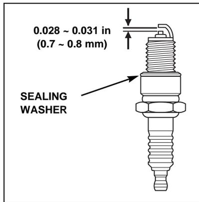
6. After the spark plug seats, tighten with a 13/16 in (21 mm) spark plug wrench to compress the washer.
