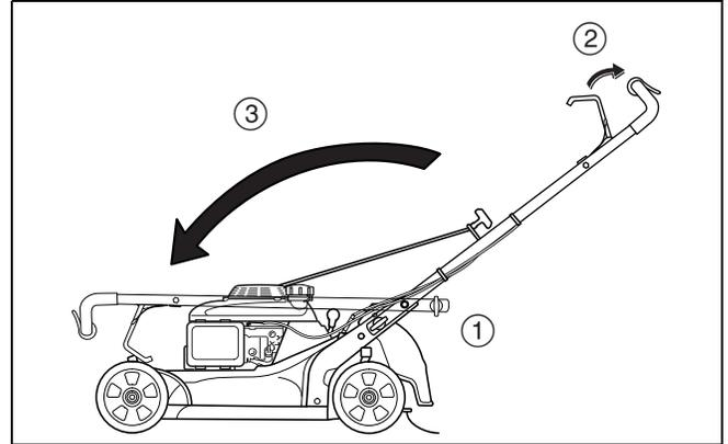
1. Turn the handlebar adjust knobs 90 degrees to release the locating pins ①.
