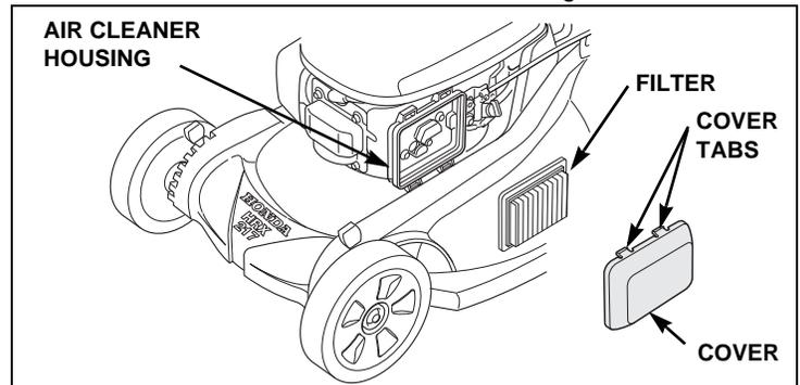
3. Inspect the filter; replace if damaged.
