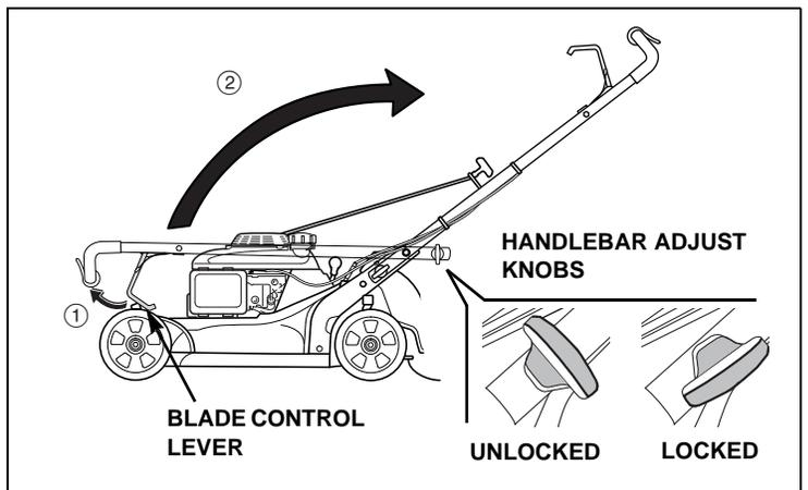
2. Align the adjust knobs with one of the three holes on each handle stay. Setting the adjust knobs to the lowest holes raises the handlebar to its highest position.
