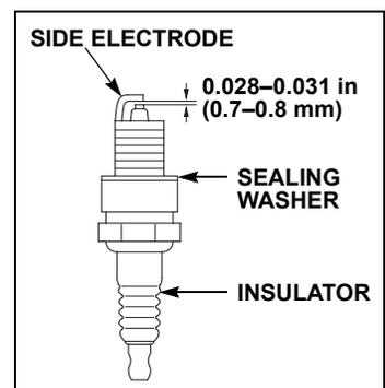
7. After the spark plug is seated, tighten with a spark plug wrench to compress the washer.
