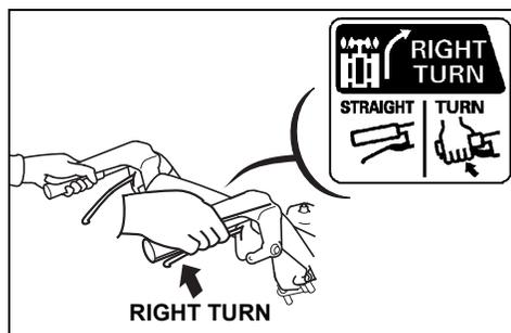
Do not partially engage or release the steering control levers. Always fully engage or fully release the levers.
