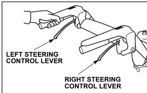
Pull the left steering control lever against the handlebar to turn the snow blower to the left.
