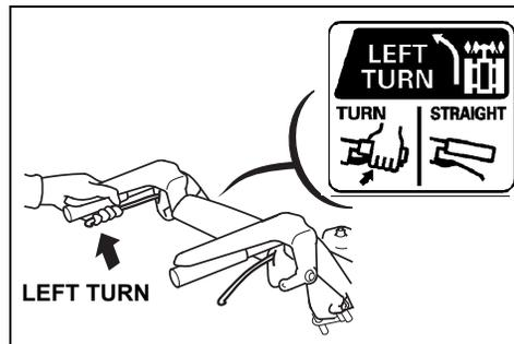
Pull the right steering control lever against the handlebar to turn the snow blower to the right.
