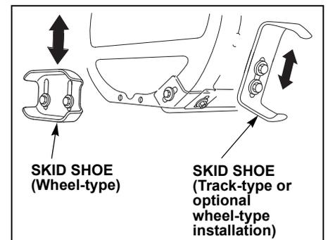
3. Loosen the skid shoe bolts and adjust the skid shoes to obtain the auger ground clearance for snow conditions recommended on the next page. Adjust the right and left skid shoes equally. Re-tighten the bolts.
