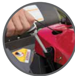
Automotive-Style Dipstick With Optimized Positioning
