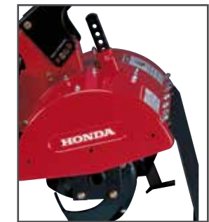
Adjustable Depth Bar This convenient feature lets you change the tilling depth.
