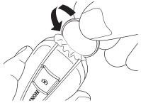
2. Replace the battery so the positive (+) and negative (-) poles are correct.
