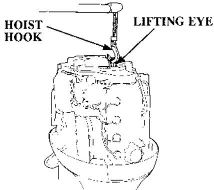
2. Hook the hoist hook to the lifting eye, and lift the motor from the boat.
