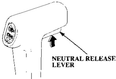
The neutral release lever is on the remote control lever to prevent an accidental gear engagement.
