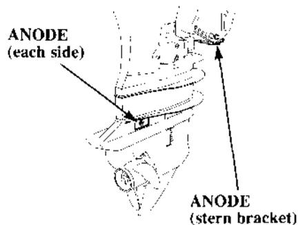
The anodes are made from a sacrificial material which helps to protect the outboard motor from corrosion.
