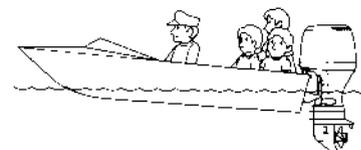
With the motor trimmed low, the trim meter will read as shown. To raise the bow, increase the motor trim angle by pressing the UP portion of the power trim/tilt switch.
