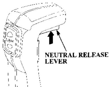
The remote control lever controls gear selection and throttle opening positions.
