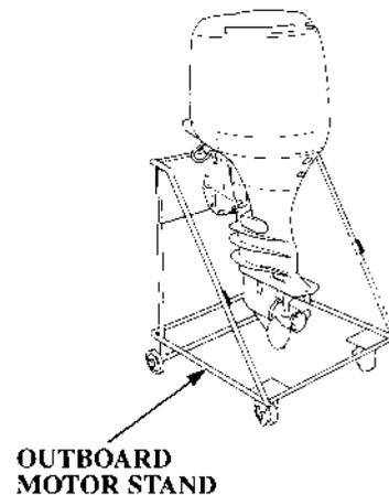
3. Place the motor on an outboard motor stand and secure with bolts and nuts.
