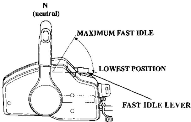
The fast idle lever provides fast idle for easy engine start up.
