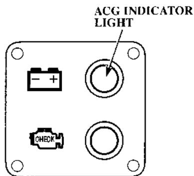
The ACG indicator light turns on and the buzzer sounds when the charging system is faulty.
