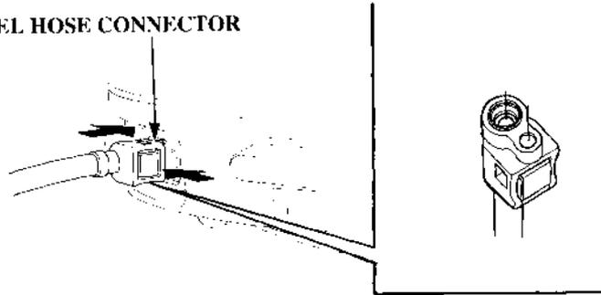
2. Connect the fuel hose connector to the outboard motor. Install the outboard end fuel hose connector with the clip toward the inside. Be sure the fuel hose connector is securely snapped in place.
