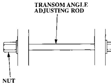
Start with the transom angle adjusting rod in the hole closest to the boat transom, lower the motor and operate the boat at full speed. If the bow is excessively low stop the boat. Tilt the motor up and raise the transom angle adjusting rod one more hole away from the transom and retest. The optimum boat trim is when the boat is parallel with the water.
