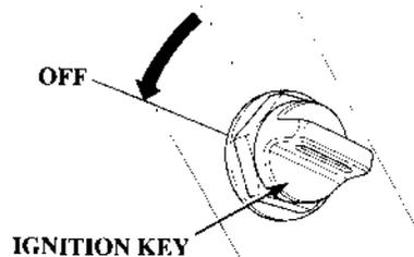
2. When the boat is not in use, remove and store the ignition switch key(s).
