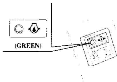
The green oil pressure indicator light turns OFF and the buzzer sounds when the oil level is low and/or the engine lubrication system is faulty. The engine speed slows down gradually.
