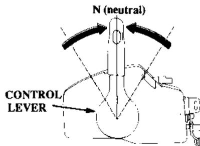
1. Move the control lever to the N (neutral) position, and turn the ignition key to the OFF position.
