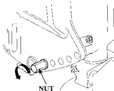
The transom angle adjusting rod limits the angle of the outboard motor when fully lowered.
