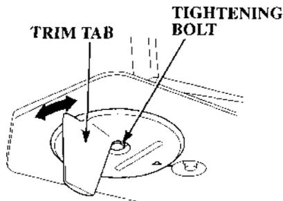
When making a turn, if an unequal amount of effort is required to turn the steering wheel right or left, adjust the trim tab so that an equal amount of effort is required.
