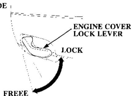
The engine cover lock levers are used to fasten the engine cover.
