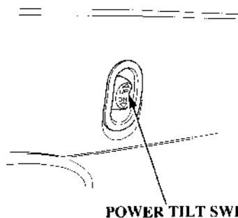
The power tilt switch located on the engine pan is a convenience switch for tilting the motor for trailering, or performing outboard motor maintenance. This power tilt switch should only be operated when the boat is stopped and the engine is off.
