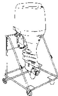
Store the motor vertically, as shown above. Store the outboard motor in a well-ventilated area free from direct sunlight and humidity.
