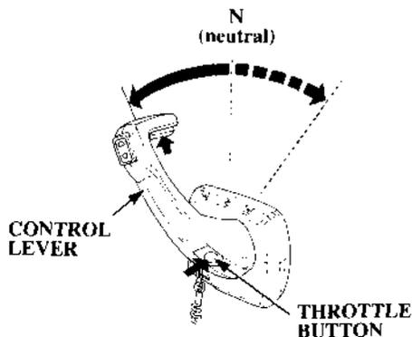
3. Push the throttle button, then move the control lever forward or backward to open the throttle slightly.
