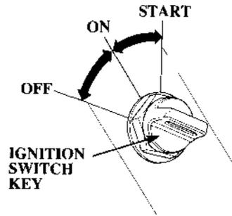
The switch panel is equipped with a key-type ignition switch.
