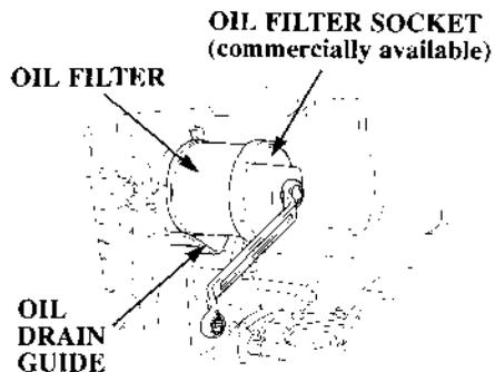
4. Clean the oil filter mounting base, and coat the gasket of the new oil filter with clean engine oil.
