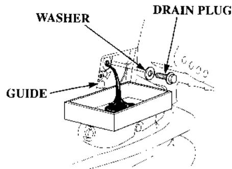
3. Place a suitable container under the guide. Remove the engine oil drain plug and washer using a 12 mm wrench, and drain the engine oil.
