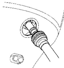
3. Connect a water hose to the water hose adapter (optional equipment), and turn on the water supply.
