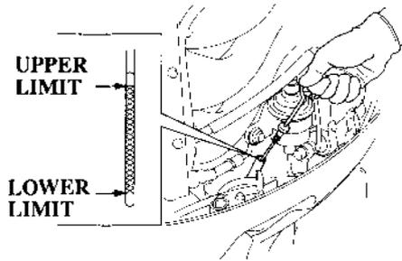
7. Inspect the engine oil level and refill to the upper limit mark on the oil level dipstick if necessary. Fill with the recommended oil.
