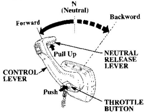
By moving the control lever forward or backward when the throttle button is pushed in, the throttle opening will be increased without engaging the gears.
