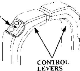
1. Press the DN portion of the power trim/tilt switch to tilt the motor to the lowest position.
