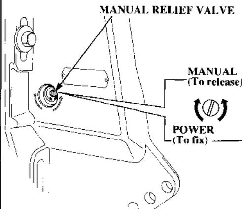
If the power trim/tilt switch will not tilt the outboard motor, the motor can be manually tilted up or down by operating the manual relief valve. To tilt the outboard motor manually, turn the manual relief valve under the left stern bracket no more than 1 or 2 turns counterclockwise, using a screwdriver.
