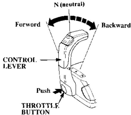
By moving the control lever forward or backward when the throttle button is pushed in, the throttle opening will be increased without engaging the gears.
