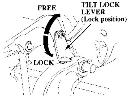
It may be necessary to lift the engine cover grip slightly to swing the tilt lock lever into the LOCK position.
