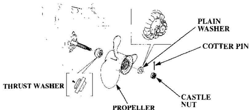
If the propeller is damaged by striking a rock, or other obstacle, replace the propeller as follows.
