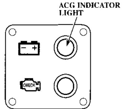
The ACG indicator light turns on and the buzzer sounds when the charging system is faulty.
