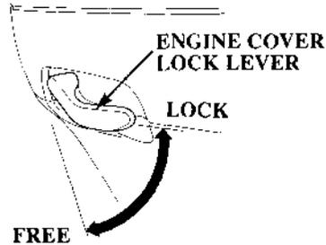
To install, position the engine cover over the engine and turn the front and side lock levers on the LOCK position.
