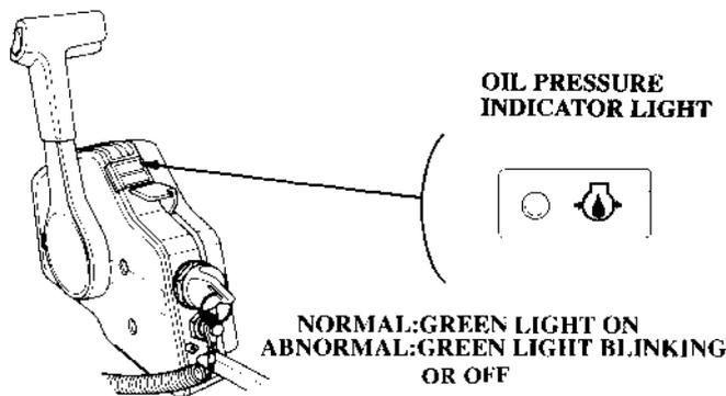
7. With the engine running, check to see if the green engine oil pressure indicator light turns ON. Stop the engine if the oil pressure indicator light does not turn ON. Check the engine oil level (see page 40). If the oil level is normal and the oil pressure indicator light does not turn ON, contact your closest authorized Honda Marine dealer.
