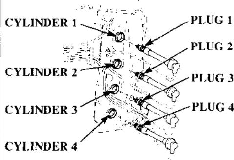
9. Reinstall the spark plug caps, matching the numbers on the cords with the cylinder numbers, as shown.
