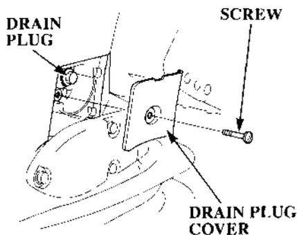
2. Remove the drain plug cover screw using a flat blade screwdriver, and remove the drain plug cover.
