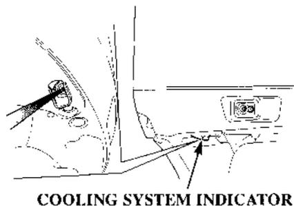
The cooling system is monitored here to make sure cooling water is circulating through the engine.
