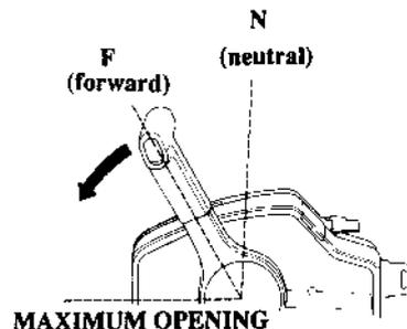
Moving the control lever farther than 30° will increase the throttle opening and boat speed.
