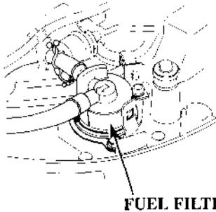
The engine fuel filter is located under the engine cover between the fuel coupling and the fuel pump. Water or sediment accumulated in the fuel filter can cause loss of power or hard starting.
