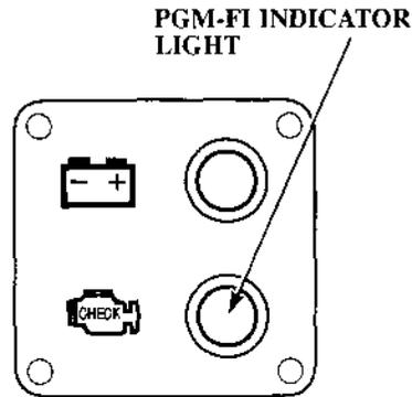
The PGM-FI indicator light turns on and the buzzer sounds when the engine control system is faulty and when the ignition key is turned from OFF to ON.
