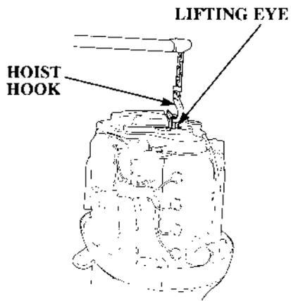
2. Hook a hoist hook to the lifting-eye, and lift the motor from the boat.
