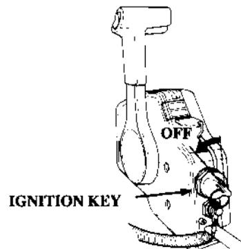
2. When the boat is not in use, remove and store the ignition key.
