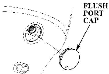
Thoroughly clean and flush the outboard motor with fresh water after operation in dirty or salty water.
