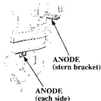
The anodes are a sacrificial material which helps to protect the outboard motor from corrosion.
