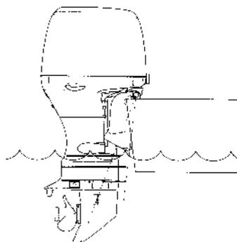
2. Move the control lever approximately 35° from N (neutral) toward F (forward) to engage the F (forward) gear.
