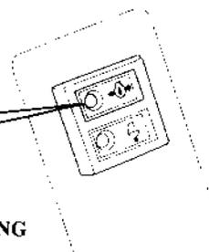
8. With the engine running, check to see if the green engine oil pressure indicator light turns ON. Stop the engine if the oil pressure indicator light does not turn ON. Check the engine oil level (see page 40). If the oil level is normal and the oil pressure indicator light does not turn ON, contact your closest authorized Honda Marine dealer.
