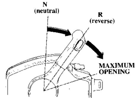
The control lever will not move unless the neutral release lever is pulled up, and the fast idle lever is in the lowest position.
