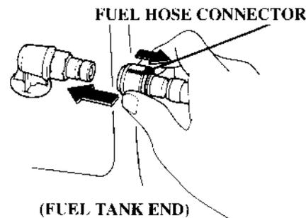
Inspect the fuel hose, and the O-ring seals in the fuel hose connectors. Replace the fuel hose, or fuel hose connectors if they are cracked, damaged or leaking fuel. Be sure the fuel hose is not kinked.
