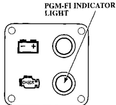
The PGM-FI indicator light turns on and the buzzer sounds when the engine control system is faulty, and when the ignition key is turned from OFF to ON.
