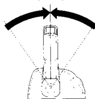
2. Move the control lever to the N (neutral) position.
