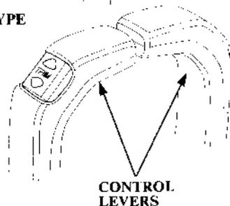
The remote control lever controls gear selection and throttle opening positions.
