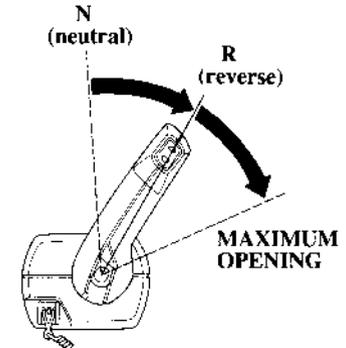
The control lever will not move unless the neutral release lever is pulled up.
