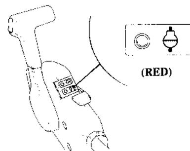
The red overheat indicator light turns ON and the buzzer sounds when there is a cooling system problem. The engine speed slows down gradually.
