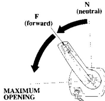
Moving the control lever farther forward or backward than 35° will increase throttle opening and boat speed.
