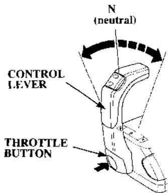
3. Push the throttle button, then move the control lever (s) forward or backward to open the throttle slightly.
