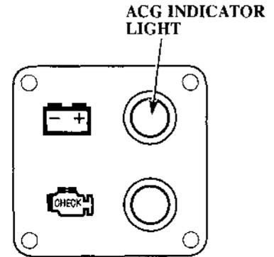
The ACG indicator light turns on and the buzzer sounds when the charging system is faulty.
