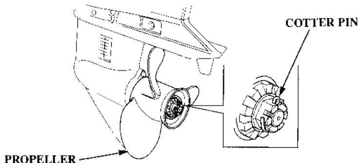
Engine speed varies according to the propeller size and the boat condition. Use of the outboard motor outside the full throttle speed range will adversely affect the engine and cause serious problems. Use of the correct propeller assures powerful acceleration, high top speed, economy and cruising comfort, and it assures longer engine life as well.
