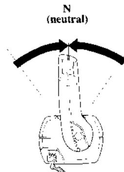
2. Move the control lever to the N (neutral) position.
