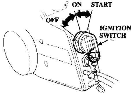
The remote control box is equipped with a key-type ignition switch. Key positions:
