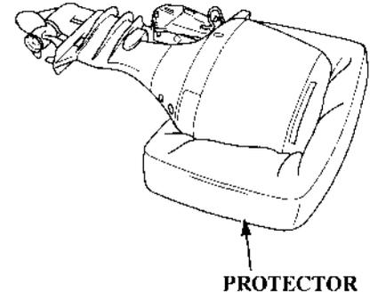
Always rest the motor on protectors, and be sure to protect it from impact and damage.
