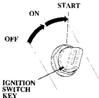
4. Turn the ignition switch key to the START position and release the key when the engine starts. The starter motor consumes a large amount of current. Do not run it continuously for more than 5 seconds at a time.
