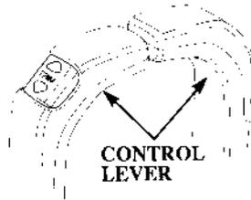
Move the control lever approximately 35° toward F (forward) or toward R (reverse) to engage the desired gear.
