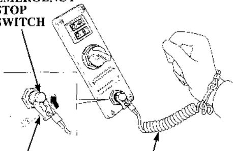
EMERGENCY STOP SWITCH LANYARD EMERGENCY STOP SWITCH CLIP
