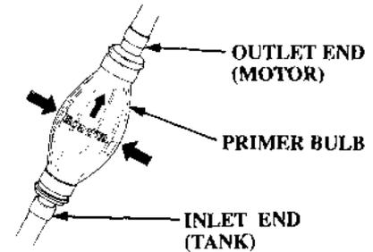
3. Hold the primer bulb so that the outlet end is higher than the inlet end. The arrow on the primer bulb points upward. Squeeze the primer bulb several times until it feels firm, indicating that fuel has reached the engine. Check for fuel leaks and repair any leaks before starting the engine.
