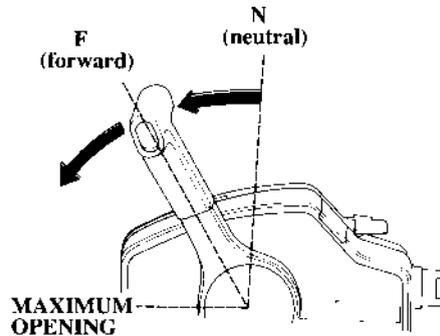
Moving the control lever farther forward or backward than 30° will increase throttle opening and boat speed.
