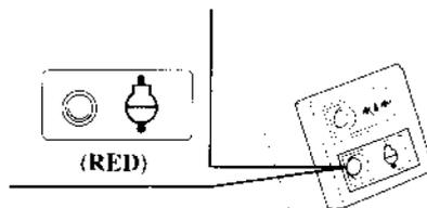
The red overheat indicator light turns ON and the buzzer sounds when there is a cooling system problem. The engine speed slows down gradually.
