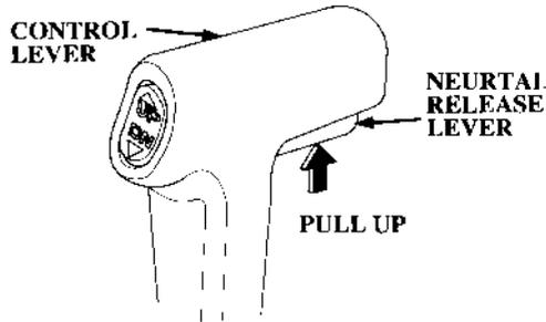
While pulling up the neutral release lever, move the control lever approximately 30° toward F (forward) or toward R (reverse) to engage the desired gear.
