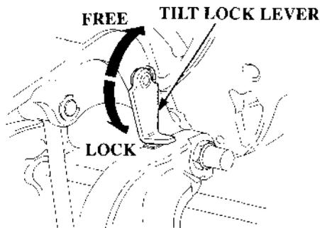
Use the tilt lock lever to hold the motor in the highest tilt position when the boat is moored for a long time.
