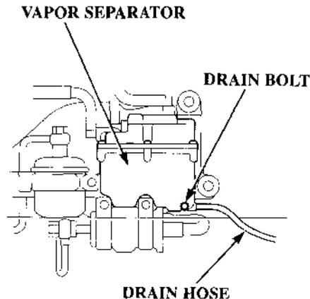
1. Remove the drain hose from the silencer case.
