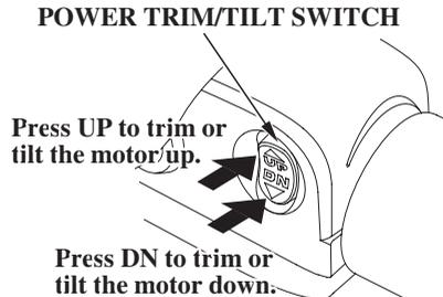
The power trim/tilt switch is located on the control lever or the tiller handle. It is a rocker switch with UP and DN (down) positions for changing the angle of the outboard motor.
