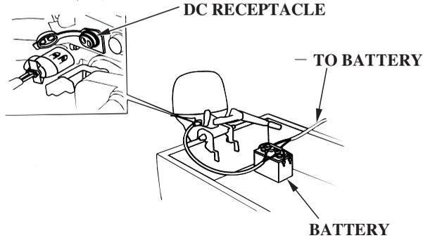
To prepare the outboard motor for connection to a battery, pull the cover out of the DC receptacle, connect your battery charging wires to the receptacle. Attach the connected DC receptacle on the holder on the tiller arm.
