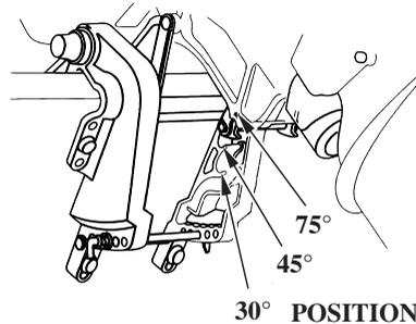
To tilt the outboard motor, move the tilt lever to the TILT position, then raise the outboard motor to the 30° or 45° position by pulling on the engine cover grip.
