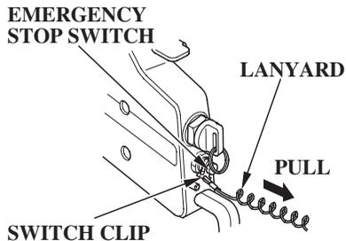
To stop the engine in an emergency, pull the clip out of the emergency stop switch by pulling the lanyard.
