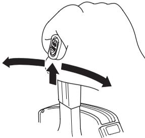
To shift gears, move the control lever to select F (forward), N (neutral) and R (reverse) gears.
