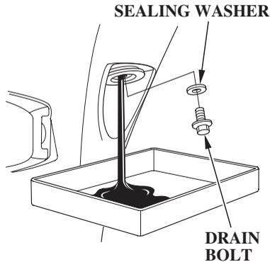
2. Remove the engine oil drain bolt and washer.
