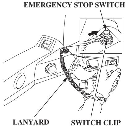
1. Put the emergency stop switch clip in the emergency stop switch, and attach the lanyard to your PFD (Personal Flotation Device) or to your wrist, as shown.
