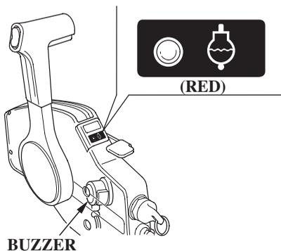
If the engine overheats, the red light will come on, and the engine protection system will limit engine speed.
