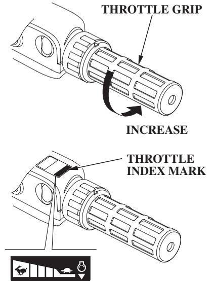
The throttle grip controls engine speed.
