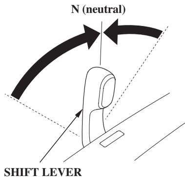
2. Check the position of the gearshift lever. It must be in the N (neutral) position for starting.
