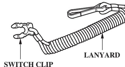
The switch clip must be inserted in the emergency stop switch in order for the engine to start and run. The lanyard must be attached to the operator's PFD (Personal Flotation Device) or worn around the wrist as shown.
