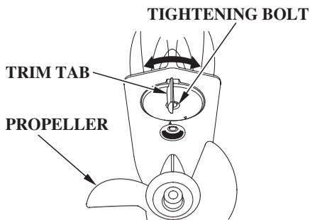
Adjust the trim tab with the engine stopped. Loosen the bolt above the trim tab, turn the trim tab, then tighten the bolt securely.
