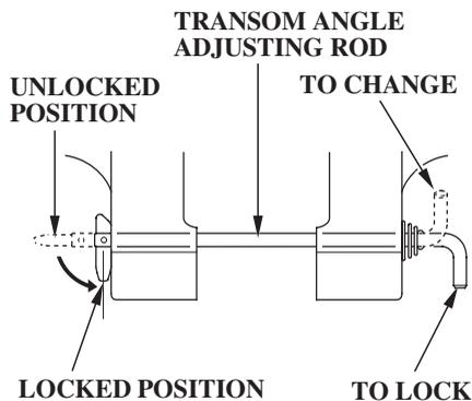
The transom angle adjusting rod limits the tilt angle of the outboard motor when fully lowered.
