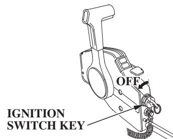
2. Turn the ignition switch key to the OFF position to stop the engine or press the emergency stop switch until the engine stops.
