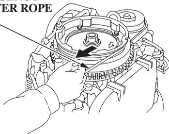
5. Pull the emergency starter rope slowly until resistance is felt, then pull briskly.
