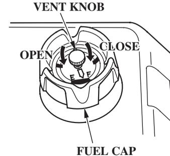
The cap is provided with a vent knob to seal the portable fuel tank for carrying it to and from the boat. Open the vent knob 2 or 3 turns before starting the engine (p. 42).
