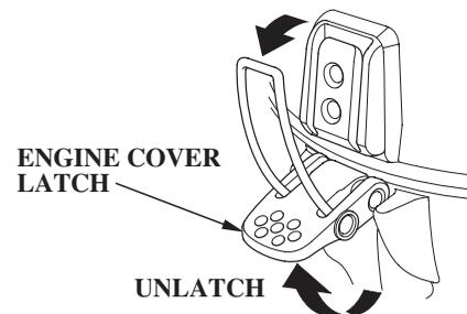
1. Unlatch and remove the engine cover.
