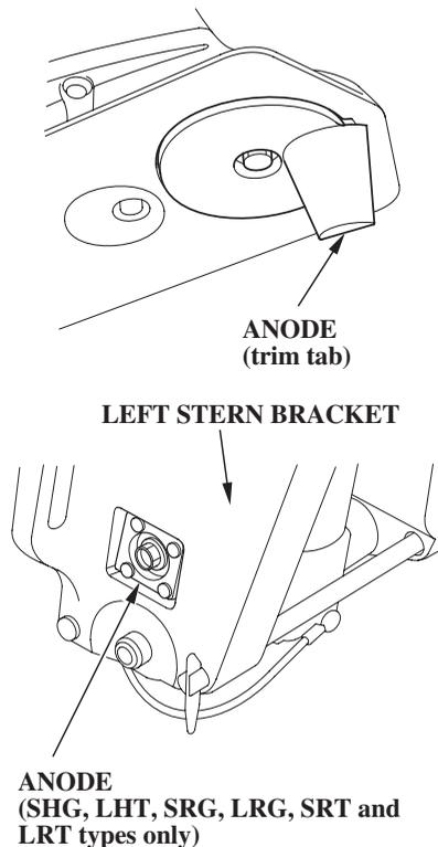
The anodes are located on the trim tab and the stern bracket. They are made of a sacrificial material that helps to protect the outboard motor from corrosion.
