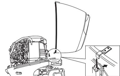
The engine cover latches fasten the engine cover to the outboard motor.
