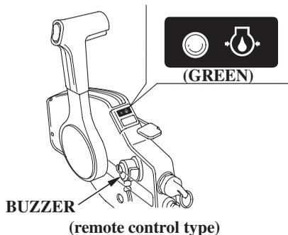
If oil pressure becomes low, the green indicator light will go off, and the engine protection system will limit engine speed. If you are at cruising speed, engine speed will decrease gradually.
