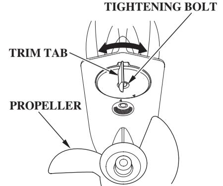
The trim tab compensates for “torque steer,” which is a reaction of the outboard motor to propeller rotation.
