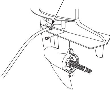
2. Remove the sealing washer from the wash plug and install the sealing washer on the flush kit coupler.
