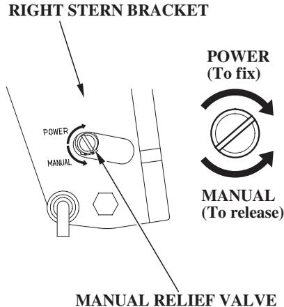
The outboard motor can be tilted manually after opening the manual relief valve. This allows the outboard motor to be tilted when no battery is connected.
