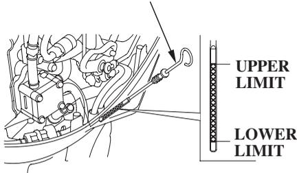
3. Insert the dipstick all the way in, then remove it and check the oil level shown on the dipstick.
