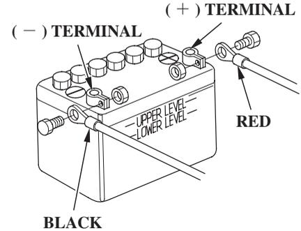
Connect the positive (+) battery cable to the positive (+) battery terminal, then connect the negative (-) battery cable to the negative (-) battery terminal.
