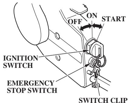
The ignition switch controls the ignition system and starter motor.
