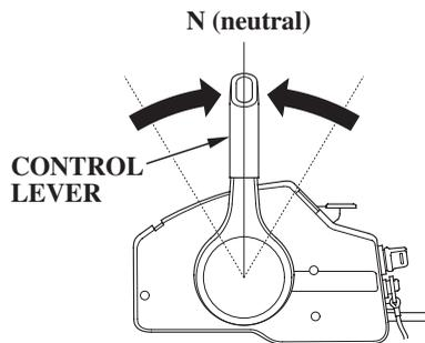
1. Move the throttle grip to the slowest speed and control gears to N (neutral) position.
