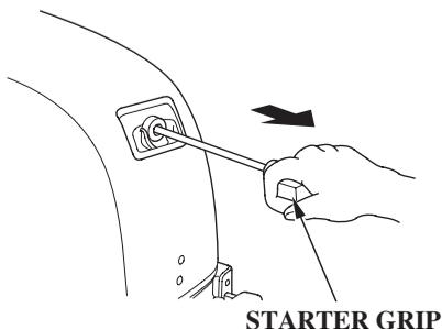
Pull the starter grip to operate the recoil starter for starting the engine manually.
