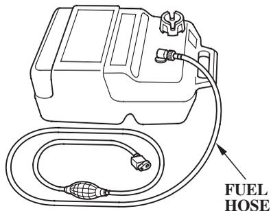
Place the portable fuel tank in a well-ventilated location, away from direct sunlight, to reduce the possibility of a gasoline vapor explosion.
