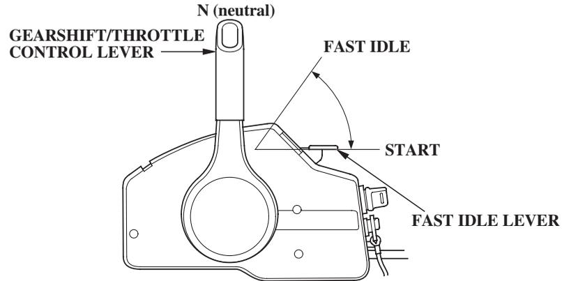
The fast idle lever is used to set idle speed during warm-up.
