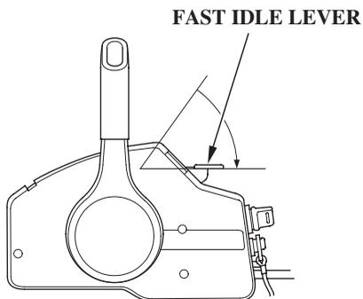
5. If the fast idle lever was used to start the engine, gradually lower the lever as the engine warms up.
