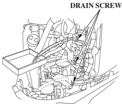
2. With the outboard motor in a vertical position, place an approved gasoline container below the fuel drain outlet, and use a funnel to avoid spilling fuel.
