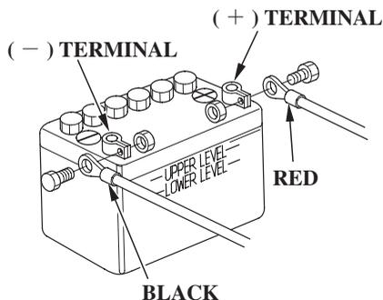
Honda BF25D and BF30D outboard motors produce a 12-volt, 4 or 10-ampere battery-charging current and are equipped for connection to a 12-volt battery. The battery-charging circuit is protected by a 15-ampere fuse located in the engine compartment.
