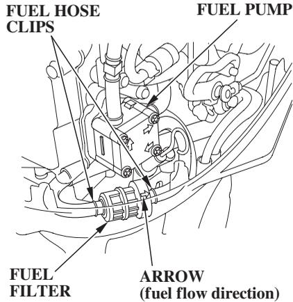
5. Install the new fuel filter so the arrow on the fuel filter points toward the fuel pump.
