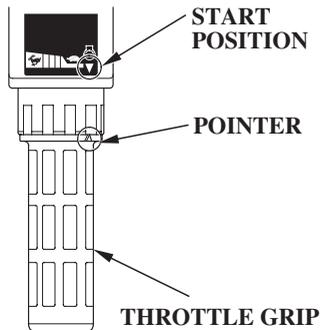
3. Align the engine start symbol "⊖" on the tiller handle with the pointer "▶" on the throttle grip.
