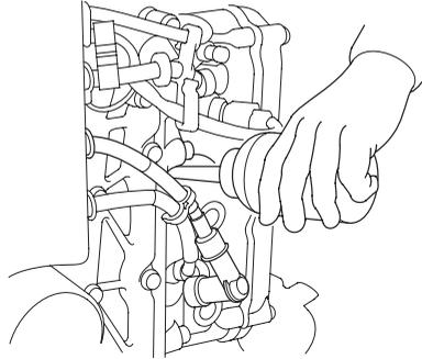
5. Pour a teaspoon of engine oil into each spark plug hole, then pull the recoil starter grip several times to lubricate the inside of the cylinders.
