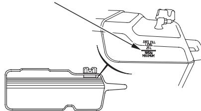
Refuel in a well-ventilated area. Fill the tank to the SAFE FILL LEVEL line.
