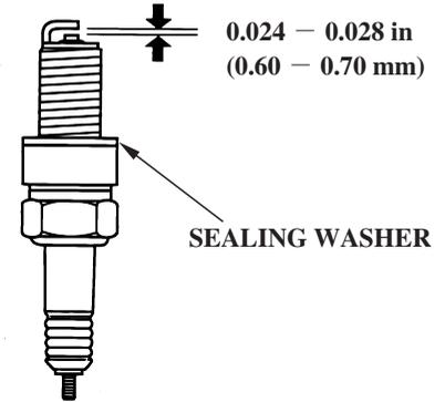
5. Measure the spark plug electrode gap with a suitable gauge. The gap should be 0.024 - 0.028 inches (0.60 - 0.70 mm).
