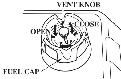
To refuel, turn the vent knob counterclockwise to the OPEN position, and unscrew the fuel tank cap.
