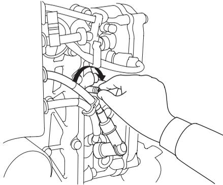
6. Install the spark plugs carefully, by hand, to avoid cross-threading.
