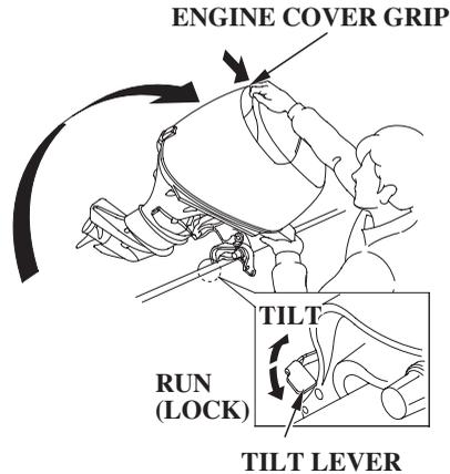
To tilt the outboard motor, move the tilt lever to the TILT position, then raise the outboard motor to the desired position by pulling on the engine cover grip.
