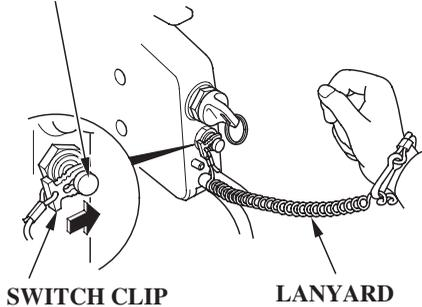
1. Put the emergency stop switch clip in the emergency stop switch, and attach the lanyard to your PFD (Personal Flotation Device) or to your wrist, as shown.
