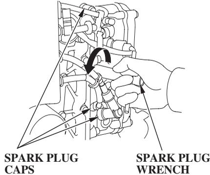
4. Inspect the spark plugs. Replace them if the electrodes are worn, or if the insulators are cracked or chipped.
