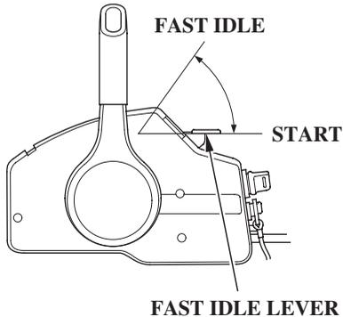
3. To start a cold engine, leave the fast idle lever in the START (fully lowered) position.
