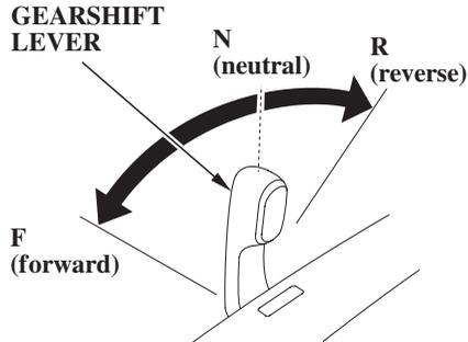
To shift gears, turn the throttle grip to the SLOW position, then move the gearshift lever to select F (forward), N (neutral) or R (reverse) gears.
