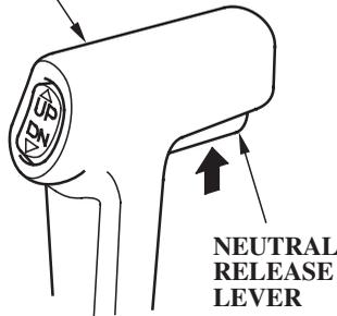
The control lever automatically locks itself in the N (neutral) position. To move the lever out of the N (neutral) position, you must squeeze the neutral release lever on the underside of the lever handle.
