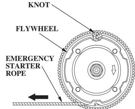
4. Set the knotted end of the emergency starter rope in the notch in the flywheel. Wind the rope clockwise around the flywheel, as shown.
