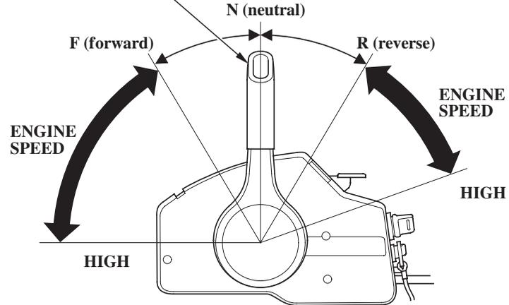
The gearshift/throttle control lever controls engine speed and selects F (forward), N (neutral), or R (reverse) gears.
