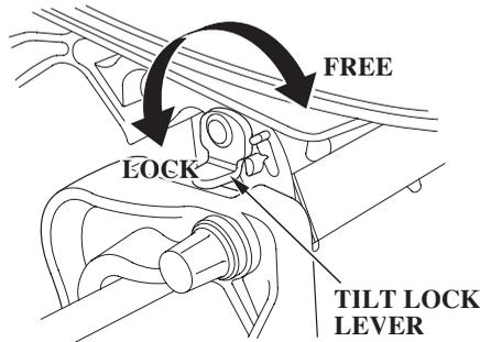
The tilt lock lever is used to support the outboard motor in the fully-raised position.
