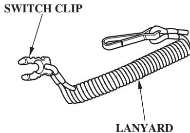
The switch clip must be inserted in the engine stop switch in order for the engine to start and run. The lanyard should be attached to the operator's PFD (Personal Flotation Device) or worn around the wrist as shown.
