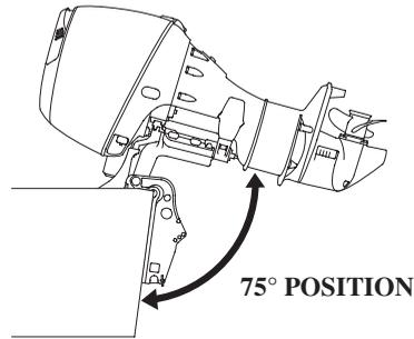
To tilt the outboard motor, move the tilt lever to the TILT position, then raise the outboard motor to the 75° position by pulling on the engine cover grip as described on p. 60.
