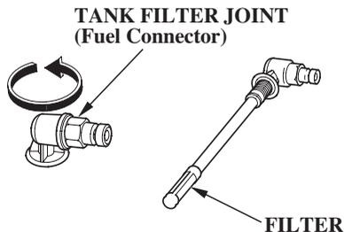
1. Unscrew the fuel hose connector by turning it counterclockwise, then remove the fuel hose connector and fuel filter from the tank.
