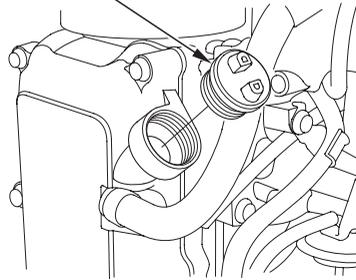
4. If the oil level is low, remove the oil filler cap, and add oil to reach the upper limit mark shown on the dipstick. Use the oil recommended on p. 73 .
