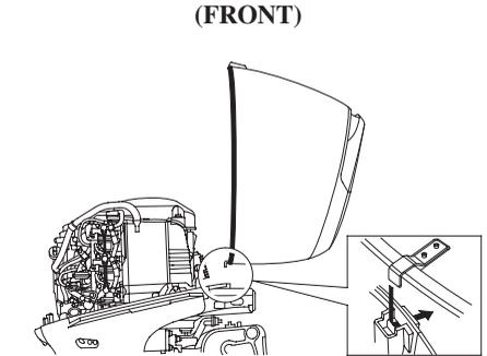
The engine cover latch fastens the engine cover to the outboard motor.
