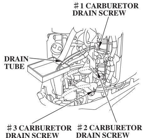
3. Loosen the drain screw on # 1 carburetor, allow the carburetor to drain completely, then tighten the drain screw securely.
