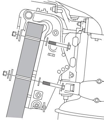
2. Secure the outboard motor with the bolts and nuts.
