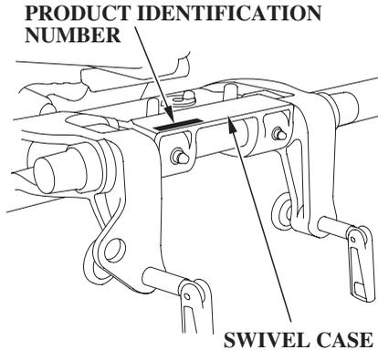
The product identification number is stamped on a plate attached on top of the swivel case.
