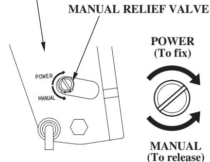
The outboard motor can also be tilted manually after opening the manual relief valve. This feature enables the outboard motor to be tilted when no battery is connected.
