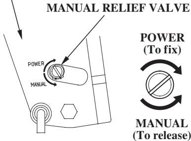
The outboard motor can be tilted manually after opening the manual relief valve. This feature enables the outboard motor to be tilted when no battery is connected.
