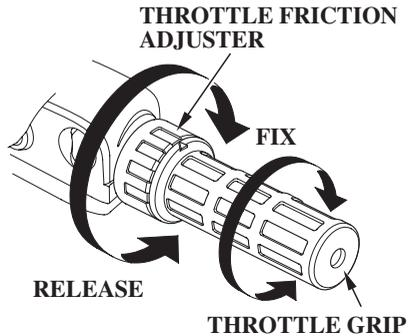
The throttle friction adjuster adjusts resistance to throttle grip rotation.
