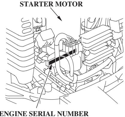
The engine serial number is stamped on the cylinder block under the starter motor which is located in the front of the engine.
