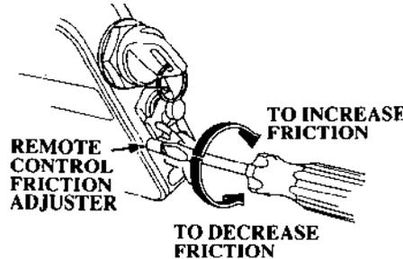
Move the remote control lever into forward and reverse gears, and check the amount of drag felt.
