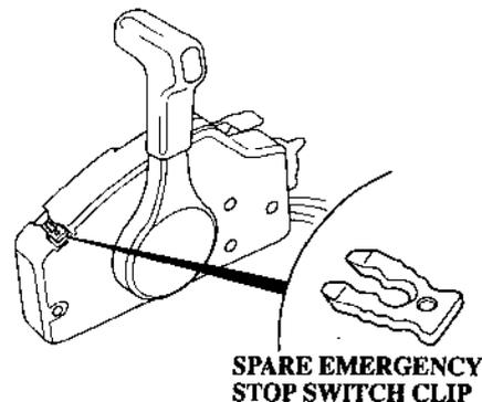
A spare emergency stop switch clip is provided on the remote control box.
