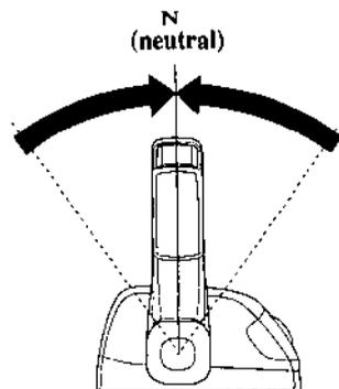
2. Move the control lever to the N (neutral) position.
