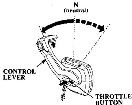
3. Move the control lever forward or backward pushing the throttle button to open the throttle slightly.
