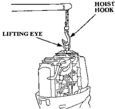
4. Hook the hoist hook to the lifting-eye, and lift the motor from the boat.
