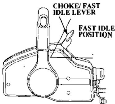
On the panel-mount and top-mount remote control type, move the control lever pushing the throttle button (not to engage the gear).
