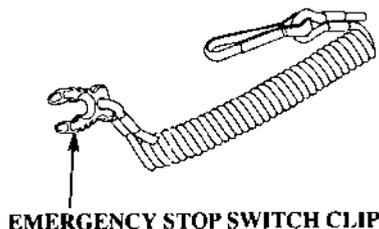
The emergency stop switch clip must be engaged with the emergency stop switch or the engine will not start. When the emergency stop switch clip becomes disengaged with the emergency stop switch, the engine will stop immediately.
