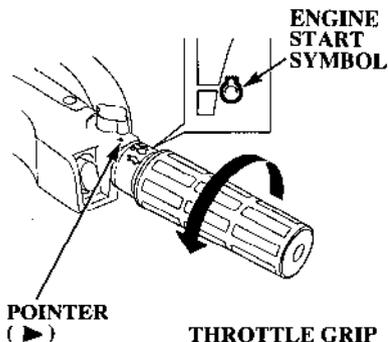
3. Align the engine start symbol "◊" on the throttle grip with the pointer "▶" on the tiller handle.
