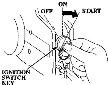
4. Holding the choke/fast idle lever in position, turn the ignition switch key to the START position, and release the key when the engine starts.
