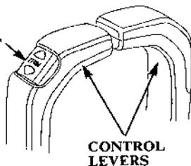
1. Press the DN portion of the power trim/tilt switch to tilt the motor to the lowest position.
