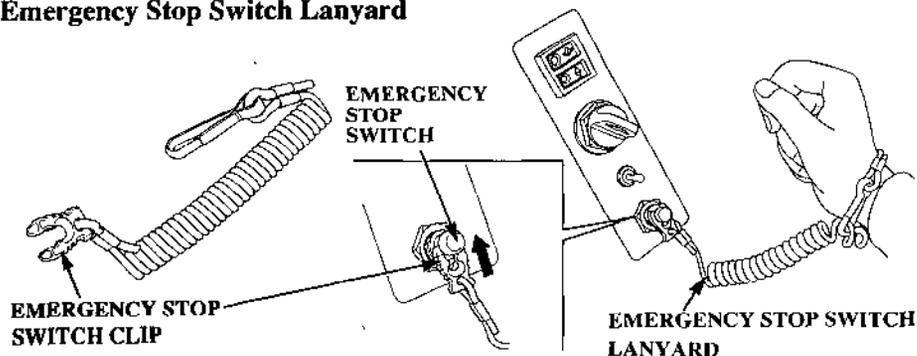
The emergency stop switch lanyard is provided to stop the engine immediately in the event the operator falls overboard or away from the controls.
