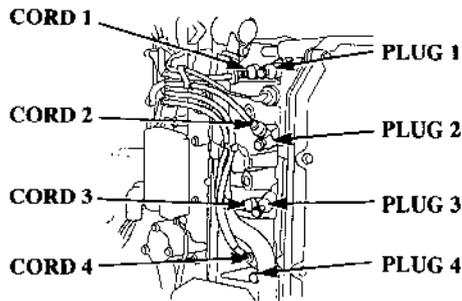
9. Reinstall the spark plug caps, matching the numbers on the cords with the cylinder numbers, as shown.
