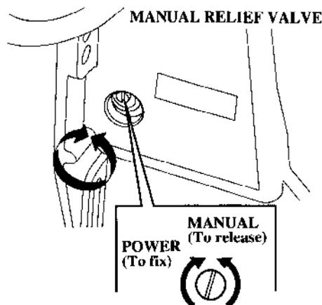
If the power trim/tilt switch will not tilt the outboard motor, the motor can be manually tilted up or down by operating the manual relief valve. To tilt the outboard motor manually, turn the manual relief valve under the left stern bracket no more than 1 or 2 turns counterclockwise, using a screw driver.
