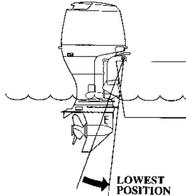
2. Move the control lever approximately 30° from N (neutral) toward F (forward) to engage the F (forward) gear.
