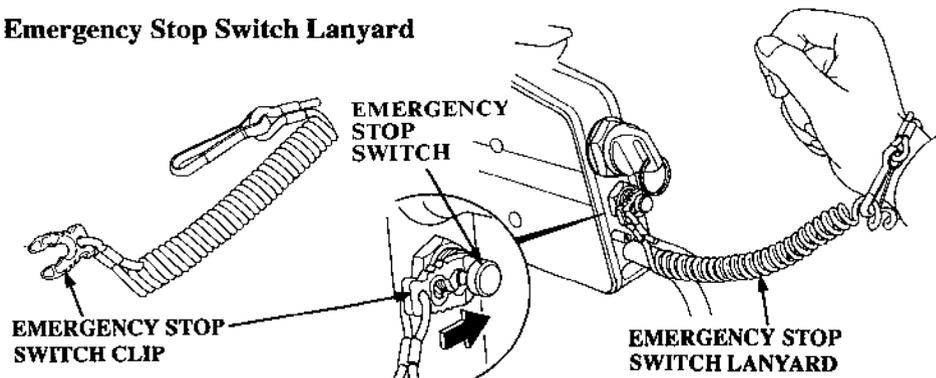
The emergency stop switch lanyard is provided to stop the engine immediately in the event the operator falls overboard or away from the controls.
