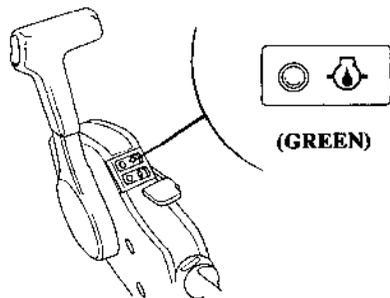
The green oil pressure indicator light turns OFF and the buzzer sounds when the oil level is low and/or the engine lubrication system is faulty. The engine speed slows down gradually.
