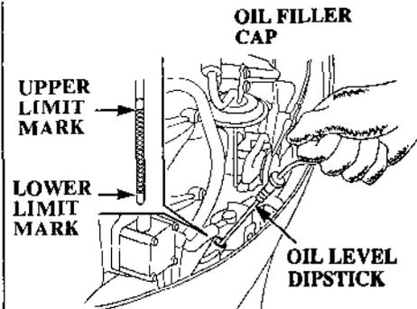
4. Reinstall the oil filler cap and tighten securely.
