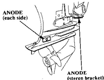
The anodes are made from a sacrificial material which helps to protect the outboard motor from corrosion.
