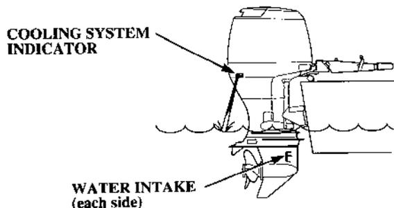
7. After the engine starts, verify water is flowing through the cooling system by monitoring the cooling system indicator. The amount of water coming out of the cooling system indicator will vary due to thermostat operation. Stop the engine if water does not come out of the cooling system indicator or if you see steam.
