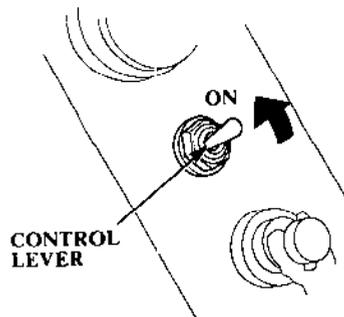
When the engine is cold, put the choke switch on. A rich fuel mixture will be provided to the engine.
