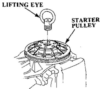
3. Install the lifting eye (optional part) onto the center of the starter pulley and tighten securely.
