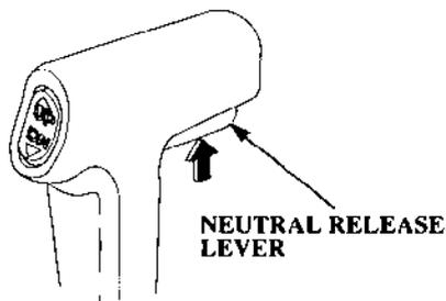
The neutral release lever is on the remote control lever to prevent an accidental gear engagement.
