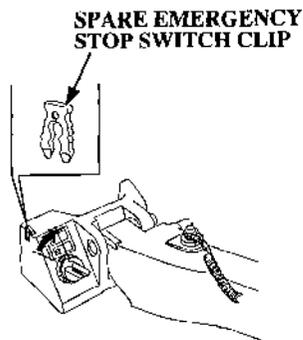
A spare emergency stop switch clip is provided near the ignition switch.
