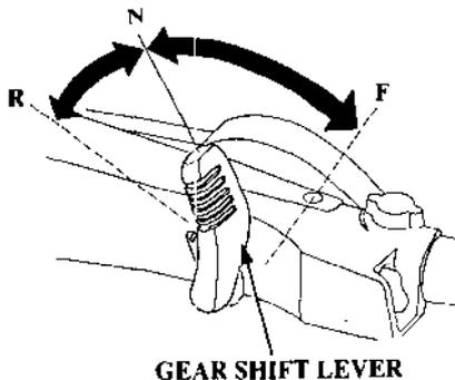
The throttle mechanism is designed to limit the throttle grip travel when operating in the **REVERSE** or **NEUTRAL** positions. The throttle grip can only be turned to the **FAST** position when operating in forward gear.
