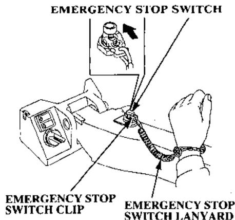
1. Engage the emergency stop switch clip (located at one end of the emergency stop switch lanyard) with the emergency stop switch.
