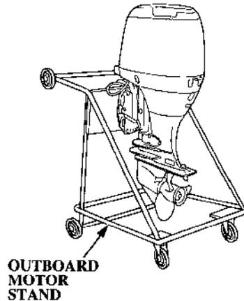
5. Place the motor on an outboard motor stand and secure with bolts and nuts.
