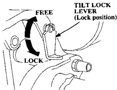
It may be necessary to lift the engine cover grip slightly to swing the tilt lock lever into the LOCK position.
