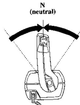
2. Move the control lever to the N (neutral) position.
