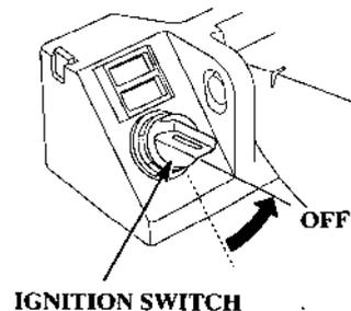
2. Turn the ignition switch to the OFF position.
