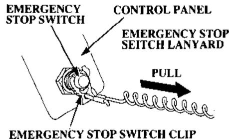
Disengage the emergency stop switch clip(s) from the emergency stop switch(es) by pulling the emergency stop switch lanyard(s).
