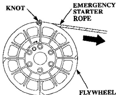
8. Set the emergency starter rope knot in the notch in the flywheel and wind the emergency starter rope counterclockwise around the flywheel.
