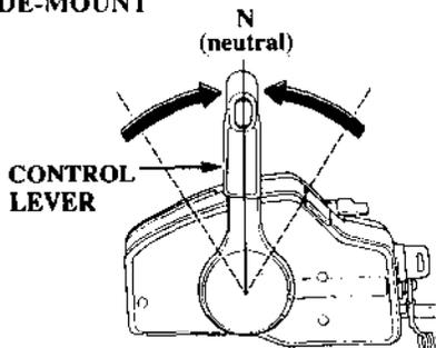
3. Depending on what type of outboard motor you have, move the shift lever or the control lever to the N (neutral) position.
