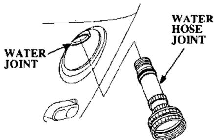
2. Install the water hose joint in the water joint.
