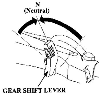
1. Turn the throttle grip to SLOW position, and move the gearshift lever to N (neutral).
