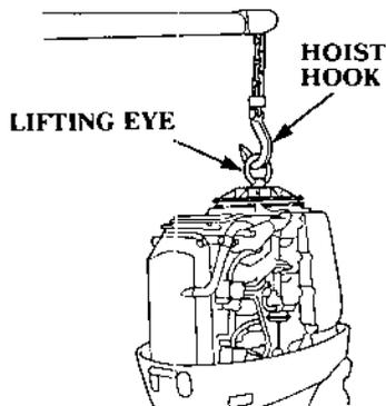
4. Hook the hoist hook to the lifting eye, and lift the motor from the boat.
