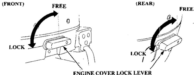
To remove, turn the front and rear engine cover lock levers to the FREE position and remove the engine cover.
