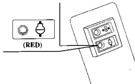
The red overheat indicator light turns ON and the buzzer sounds when there is a cooling system problem. The engine speed slows down gradually.
