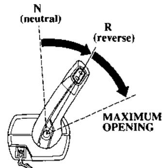
The control lever will not move unless the neutral release lever is pulled up.
