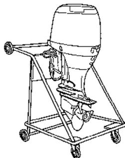
Store the motor vertically, as shown above. Store the outboard motor in a well-ventilated area free from direct sunlight and humidity.
