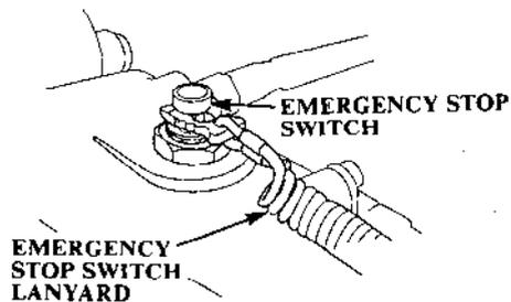
The emergency stop switch lanyard is provided to stop the engine immediately in the event the operator should fall overboard or away from the controls.
