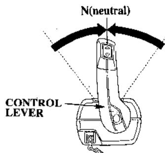
1. Move the control lever to the N (neutral) position, and turn the ignition key to the OFF position.
