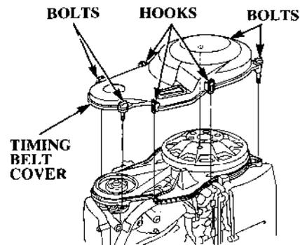
2. Loosen the four bolts and the three hooks, then remove the flywheel cover.
