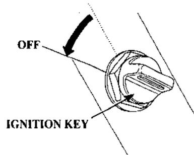
2. When the boat is not in use, remove and store the ignition switch key(s).
