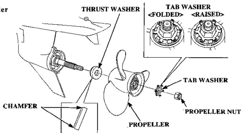
If the propeller is damaged, replace it as follows:
