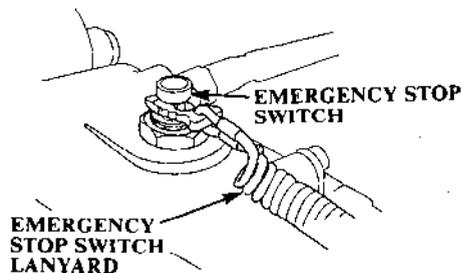
The emergency stop switch lanyard is provided to stop the engine immediately in the event the operator should fall overboard or away from the controls.
