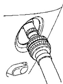
3. Connect a water hose to the water hose joint, and turn on the water supply.
