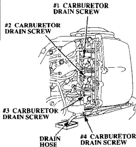
1. Remove the engine cover and disconnect the fuel hose connector.
