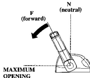
Moving the control lever farther than 35° will increase the throttle opening and boat speed.
