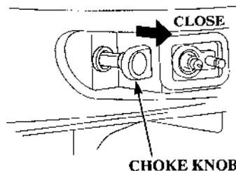
4. When the engine is cold or ambient temperature is low pull the choke knob.
