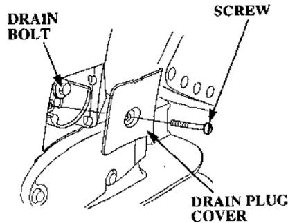
2. Loosen the drain plug cover screw using a flat blade screwdriver and remove the drain plug cover.
