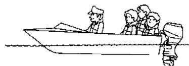
With the motor trimmed low, the trim meter will read as shown. To raise the bow, increase the motor trim angle by pressing the UP portion of the power trim/tilt switch.
