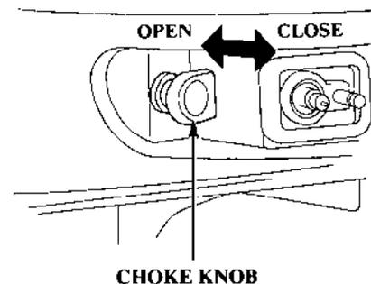
When the engine is cold, pull the choke knob. A rich fuel mixture is provided to the engine by pulling the choke knob.
