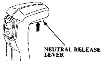
The neutral release lever is on the remote control lever to prevent an accidental gear engagement.
