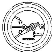
With the motor trimmed high, the trim meter will read as shown. To lower the bow, decrease the motor trim angle by pressing the DN portion of the power trim/tilt switch.
