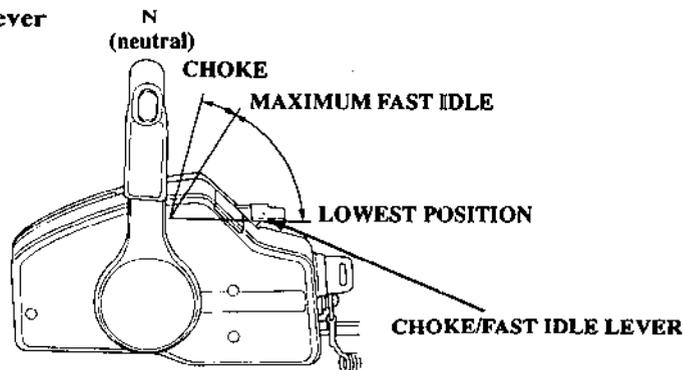
The choke/fast idle lever provides two functions:
