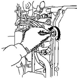
7. Thread the plugs in by hand to prevent cross threading.
