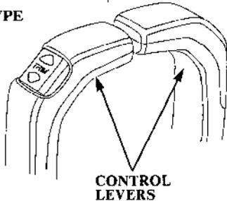
The remote control lever controls gear selection and throttle opening positions.
