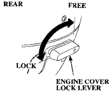
The engine cover lock levers are used to fasten the engine cover.
