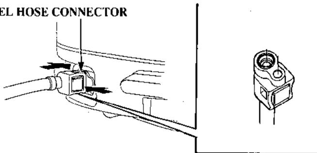
2. Connect the fuel hose connector to the outboard motor. Install the outboard end fuel hose connector with the clip toward the outside. Be sure the fuel hose connector is securely snapped in place.
