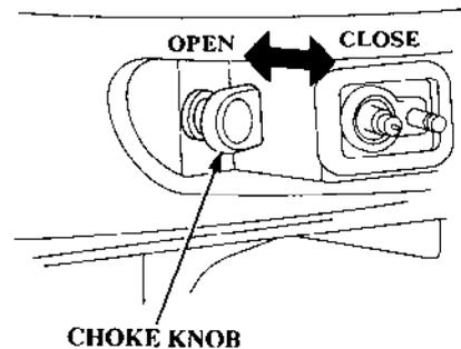
A manual choke knob is located on the right side of the motor, which can be used in the event the battery is discharged. Pull the manual choke knob, and a rich fuel mixture will be provided to the engine.
