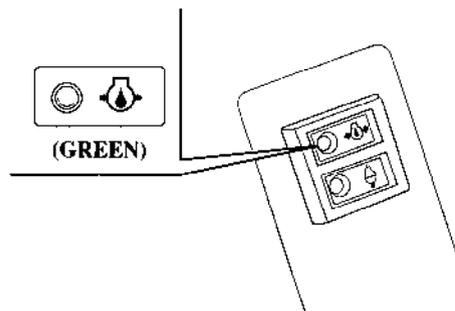
The green oil pressure indicator light turns OFF and the buzzer sounds when the oil level is low and/or the engine lubrication system is faulty. The engine speed slows down gradually.
