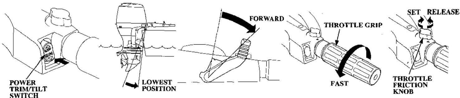
1. Press the DN portion of the power trim/tilt switch to tilt the motor to the lowest position.
