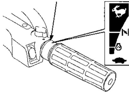
The curve on the grip label indicates throttle opening.
