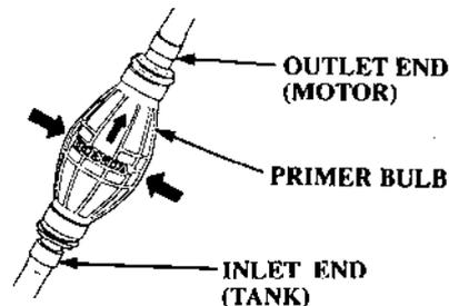
3. Hold the primer bulb so that the outlet end is higher than the inlet end. The arrow on the primer bulb points upward. Squeeze the primer bulb several times until it feels firm, indicating that fuel has reached the carburetors. Check for fuel leaks and repair any leaks before starting the engine.
