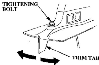
When making a turn, if an unequal amount of effort is required to turn the steering wheel or tiller handle right or left, adjust the trim tab so that an equal amount of effort is required.
