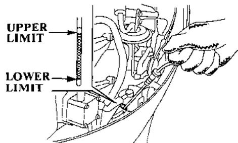
7. Inspect the engine oil level and refill to the upper limit mark on the oil level dipstick if necessary. Fill with the recommended oil.
