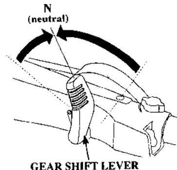
2. Move the gearshift lever to the N (neutral) position.
