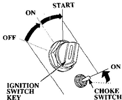
5. Holding the choke switch in position (ON), turn the ignition switch key to the START position and release the key when the engine starts. The starter motor consumes a large amount of current. Do not run it continuously for more than 5 seconds at a time.
