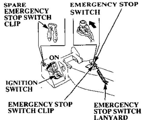
4. If your outboard motor is a tiller handle type, engage the emergency stop switch clip (located at one end of the emergency stop switch lanyard) with the emergency stop switch. Turn the ignition switch key to the ON position.
