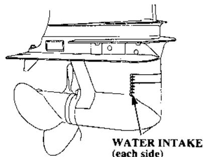
The engine cooling water is drawn into the water pump through these water intakes.
