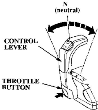
3. Move the control lever(s) forward or backward pushing the throttle button to open the throttle slightly.
