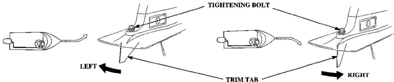
The trim tab is provided to adjust for "torque steer" which is a reaction of the propeller rotation or propeller torque. If during a high speed turn, an unequal amount of effort is required to turn the boat right or left, adjust the trim tab so that an equal amount of effort is required.
