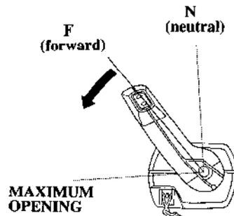
Moving the control lever farther than 35° will increase the throttle opening and boat speed.
