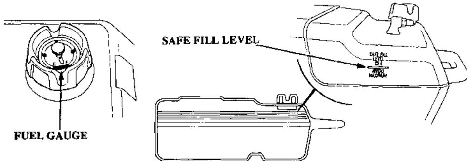
Check the fuel gauge and refill the tank to the SAFE FILL level mark if necessary.
