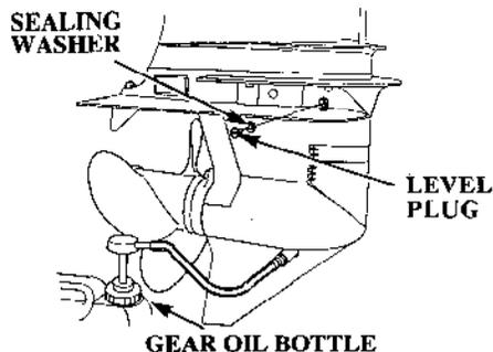
5. Disconnect the oil pump hose, and install the drain plug to avoid losing more than 1 fl oz (30 cc) of oil while reinstalling the drain plug.
