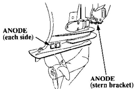
The anodes are a sacrificial material which helps to protect the outboard motor from corrosion.
