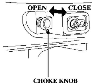
When the engine is cold, pull the choke knob. A rich fuel mixture is provided to the engine by pulling the choke knob.
