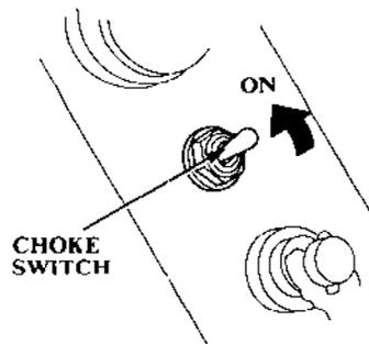
When the engine is cold, put the choke switch "ON". A rich fuel mixture will be provided to the engine.
