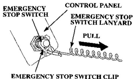
Disengage the emergency stop switch clip from the emergency stop switch by pulling the emergency stop switch lanyard.
