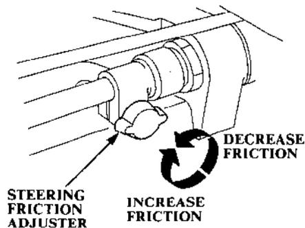
The steering friction adjuster adjusts the tightness of the steering movement.
