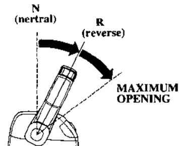
Moving the control lever farther forward or backward than 35° will increase throttle opening and boat speed.
