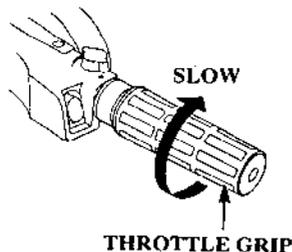
6. If it was necessary to use the choke knob to start the engine, slowly return it to its initial position. Turn the throttle grip in the SLOW direction to a position where the engine does not stall.
