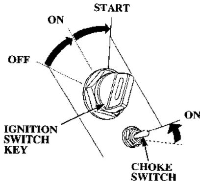
5. Holding the choke switch in the ON position, turn the ignition switch key to the **START** position and release the key when the engine starts. The starter motor consumes a large amount of current. Do not run it continuously for more than 5 seconds at a time.
