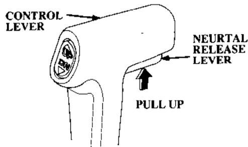
While pulling up the neutral release lever, move the control lever approximately 30° toward F (forward) or toward R (reverse) to engage the desired gear.
