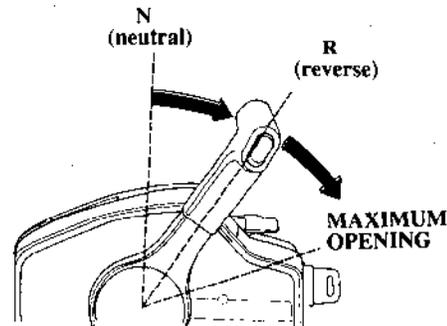
The control lever will not move unless the neutral release lever is pulled up, and the choke/fast idle lever is in the lowest position.
