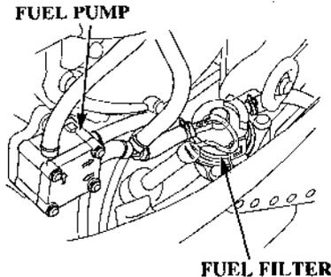
The engine fuel filter is located under the engine cover between the fuel coupling and the fuel pump. Water or sediment accumulated in the fuel filter can cause loss of power or hard starting.
