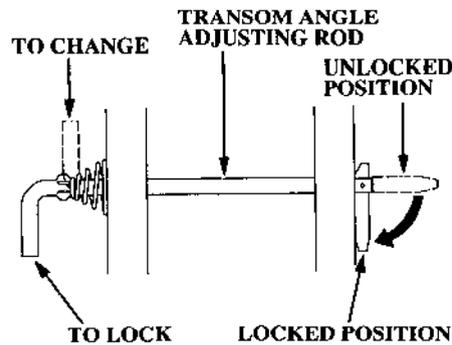
Start with the transom angle adjusting rod in the hole closest to the boat transom, lower the motor and operate the boat at full speed. If the bow is excessively low stop the boat. Tilt the motor up and raise the transom angle adjusting rod one more hole away from the transom and retest. The optimum boat trim is when the boat is parallel with the water. The transom angle adjusting rod stops, the motor's forward movement.
