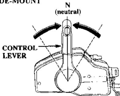
3. Depending on what type of outboard motor you have, move the shift lever or the control lever to the N (neutral) position.
