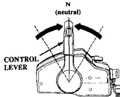
2. Move the control lever to the N (neutral) position.
