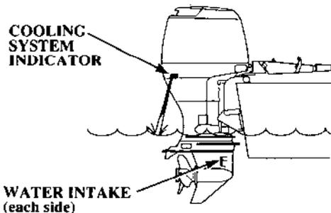
Check the water intake screens and the cooling system indicator discharge port, and if necessary remove any obstructions. If the problem continues, contact your closest authorized Honda Marine dealer.
