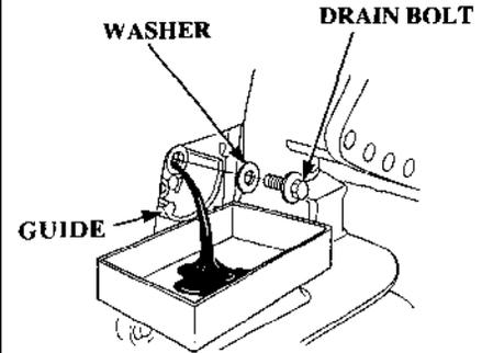
3. Place a suitable container under the guide. Remove the engine oil drain bolt and washer using a 12 mm wrench, and drain the engine oil.
