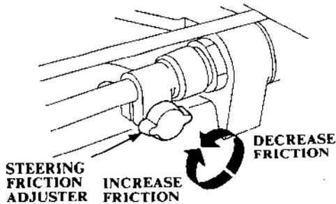
Operate the tiller handle right and left to check the tightness.
