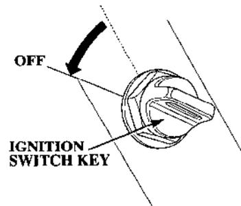
2. When the boat is not in use, remove and store the ignition key.
