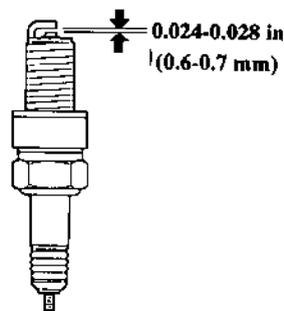
6. Measure the plug gaps with a spark plug gap gauge.
