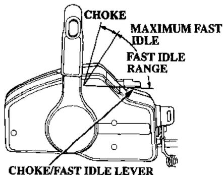
3. When the engine is cold or the ambient temperature is low, lift the choke/fast idle lever up fully. This will provide a rich fuel mixture.
