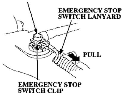
Disengage the emergency stop switch clip from the emergency stop switch by pulling the emergency stop switch lanyard.
