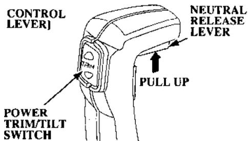
While pulling up the neutral release lever, move the control lever approximately 35° toward F (forward) or toward R (reverse) to engage the desired gear.
