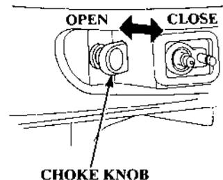
A manual choke knob is located on the right side of the motor, which can be used in the event the battery is discharged. Pull the manual choke knob, and a rich fuel mixture will be provided to the engine.
