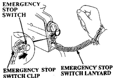
1. Engage the emergency stop switch clip (located at one end of the emergency stop switch lanyard) with the emergency stop switch.
