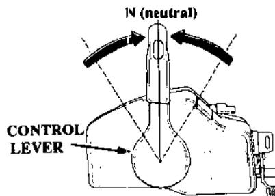
1. Move the control lever to the N (neutral) position, and turn the ignition key the OFF position.
