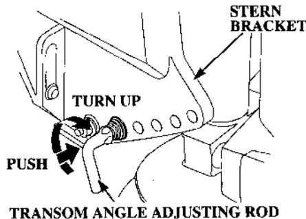
The transom angle adjusting rod is used to adjust the motor angle to achieve the correct boat trim. There are 5 adjustment holes located in the stern bracket.
