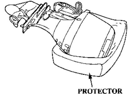
Always rest the motor on protectors and be sure to protect it from impact and damage.
