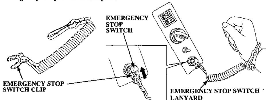
The emergency stop switch lanyard is provided to stop the engine immediately in the event the operator falls overboard or away from the controls.
