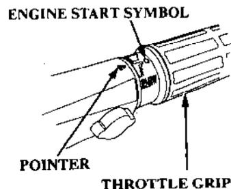
7. On the tiller handle type, align the engine start symbol "⚙" on the throttle grip with the pointer "▶" on the tiller handle.
