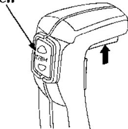
1. Press the DN portion of the power trim/tilt switch to tilt the motor to the lowest position.
