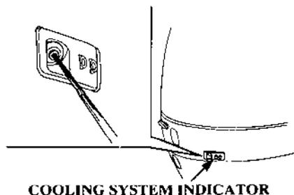
The cooling system is monitored here to make sure cooling water is circulating through the engine.
