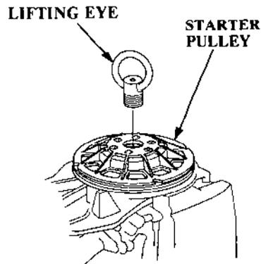
3. Install the lifting eye (optional part) in the center of the starter pulley and tighten securely.
