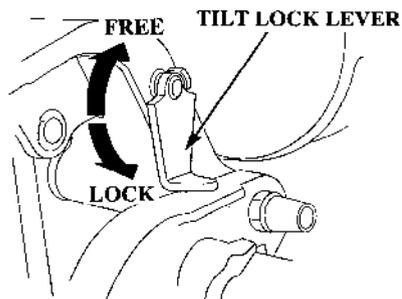
Use the tilt lock lever to hold the motor in the highest tilt position when the boat is moored for a long time.
