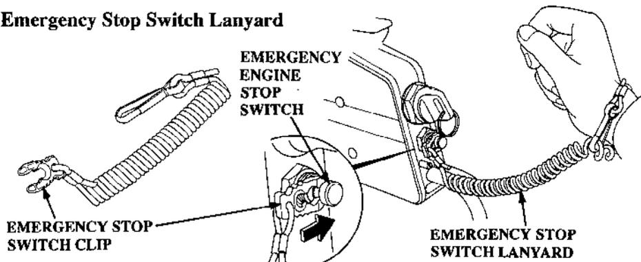
The emergency stop switch lanyard is provided to stop the engine immediately in the event the operator should fall overboard or away from the controls.
