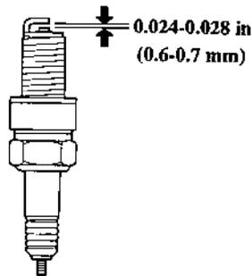
6. Measure the plug gaps with a feeler gauge. The gaps should be 0.024-0.028 in (0.6-0.7 mm). Correct as necessary by carefully bending the side electrode.
