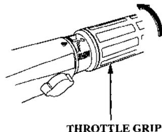
7. If it was necessary to use the choke knob to start the engine, slowly return it to its initial position. Turn the throttle grip in the SLOW direction to a position where the engine does not stall.
