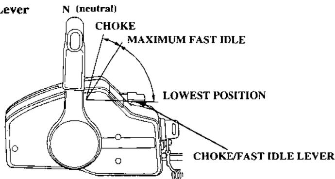
The choke/fast idle lever provides two functions:
