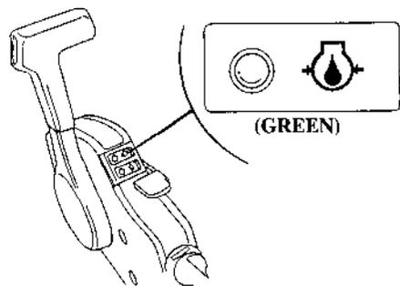
The green oil pressure indicator light turns OFF and the buzzer sounds when the oil level is low and/or the engine lubrication system is faulty.
