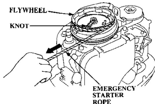
10. Set the emergency starter rope knot in the notch in the flywheel and wind the emergency starter rope clockwise around the flywheel.
