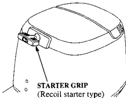
Pull the starter grip to start the engine. Set the gearshift lever in the N (neutral) position before starting. The engine will not start unless the gearshift lever is in the N (neutral) position.
