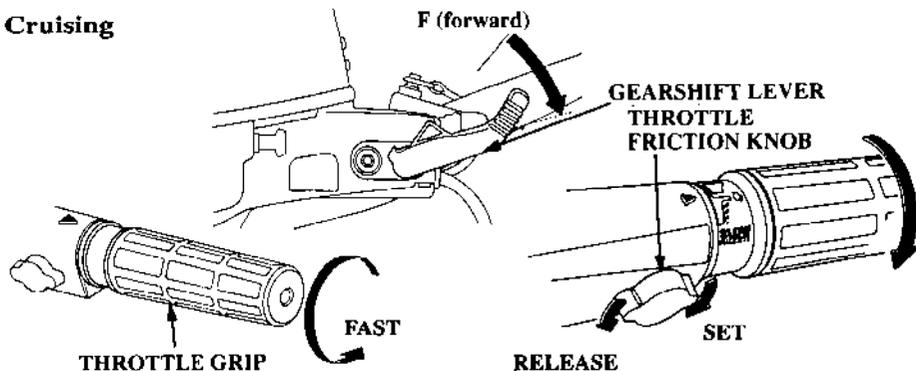
With the gearshift lever in the F (forward) position, turn the throttle grip toward the FAST mark to increase speed. For optimum fuel economy, limit throttle opening to  $2/3$ .
