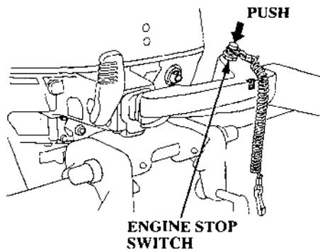
2. Push the engine stop switch until the engine stops.
