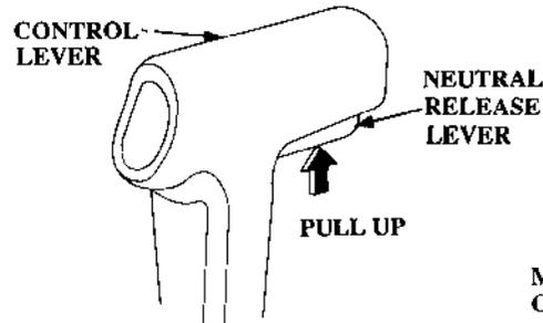
While pulling up the neutral release lever, move the control lever 30° toward F (forward) or 30° toward R (reverse) to engage the desired gear.
