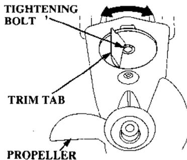
When making a turn, if an unequal amount of effort is required to turn the steering wheel or tiller handle right or left, adjust the trim tab so that an equal amount of effort is required.
