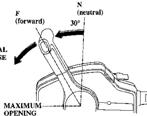
Moving the control lever further from 30° will increase throttle opening and boat speed.
