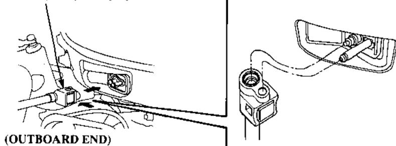
2. Connect the fuel hose connector to the outboard motor. Install the outboard end fuel hose connector with the clip toward the outside. Be sure the fuel hose connector is securely snapped in place.
