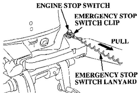
Disengage the emergency stop switch clip from the engine stop switch by pulling the emergency stop switch lanyard.
