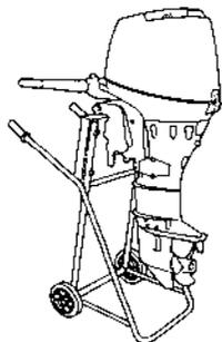
Transport and store the motor either vertically or horizontally, as shown above. Store the outboard motor in a well-ventilated area free from direct sunlight and humidity.
