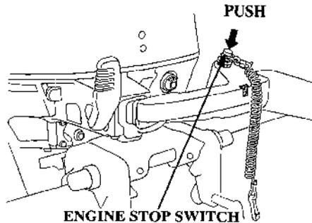
Push the engine stop switch to stop the engine.
