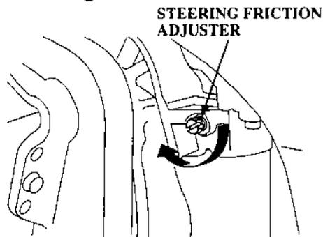
When trailering or transporting the boat with the motor attached, it is recommended that the motor remain in the normal run position. Tighten the steering friction adjuster securely to stop the motor's side to side movement.
