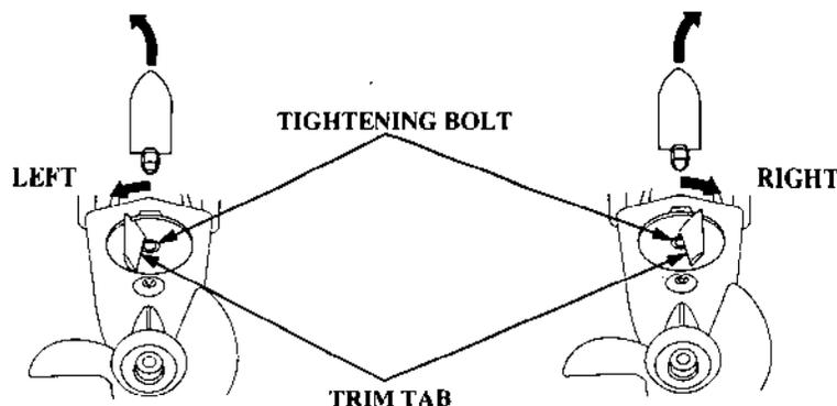
The trim tab is provided to adjust for "torque steer" which is a reaction of the propeller rotation or propeller torque. If during a high speed turn an unequal amount of effort is required to turn the boat right or left, adjust the trim tab so that an equal amount of effort is required.
