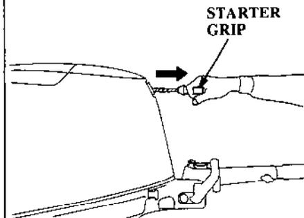
5. Pull the starter rope slowly until a resistance is felt, then pull briskly.
