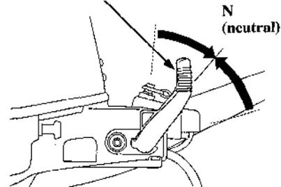
2. Move the gearshift lever to the N (neutral) position.
