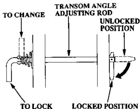
som, lower the motor and operate the boat at full speed. If the bow is excessively low stop the boat and motor. Tilt the motor up and raise the transom angle adjusting rod one more hole away from the transom and retest. The optimum boat trim is when the boat is parallel with the water. The transom angle adjusting rod stops the motors forward movement.
