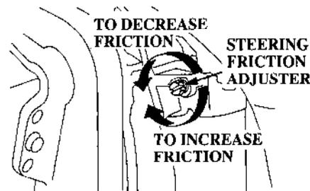
Operate the steering wheel or tiller handle right and left and check for the amount of drag felt.
