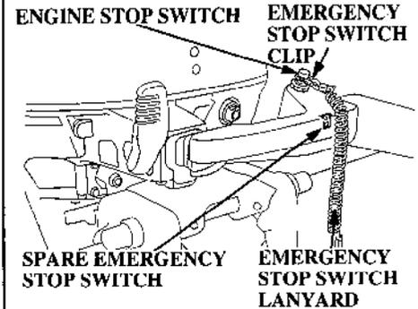
6. If your outboard motor is a tiller handle type, engage the emergency stop switch clip, located at one end of the emergency stop switch lanyard, with the engine stop switch.
