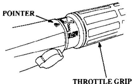
3. Align the engine start symbol "⊕" on the throttle grip with the pointer "▶" on the tiller handle.
