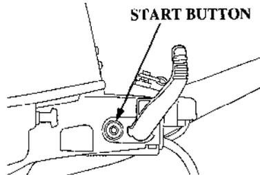
6. Press the start button and start the engine. The starter motor consumes a large amount of current. Do not run it continuously for more than 5 seconds at a time. If the engine does not start within 5 seconds wait at least 10 seconds before using the starter motor again.
