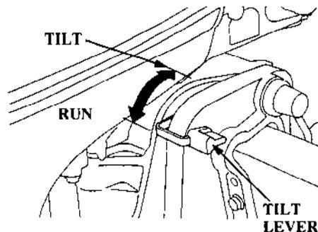
Use the tilt lever to temporarily tilt the motor when the boat is operating or mooring in shallow water.
