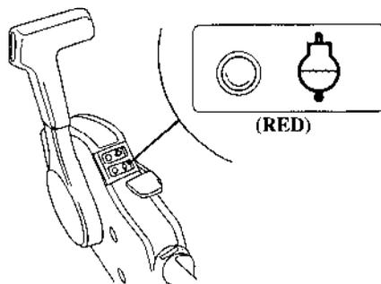
The red overheat indicator light turns ON and the buzzer sounds when the engine cooling system is faulty. The engine speed slows down gradually.
