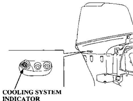
7. Start the engine. Monitor the cooling system indicator. Stop the engine if water does not come out of the cooling system indicator and check the fresh water supply. If the fresh water supply is insufficient it may be necessary to temporarily cover the three water intakes with duct tape.
