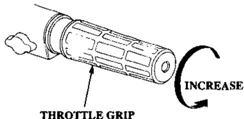
Turn the grip clockwise or counterclockwise to adjust the engine speed. Turning the grip in the direction shown by the arrow increases engine speed.
