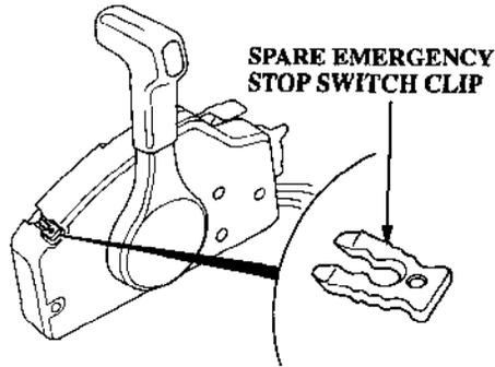
**WARNING** If the operator does not attach the emergency stop switch lanyard, and is thrown from his seat or out of the boat, the out-of-control boat can seriously injure the operator, passengers, or bystanders. Always properly attach the lanyard before starting the motor.
