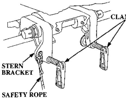
Attach the stern bracket to the transom and tighten the clamp screws.
