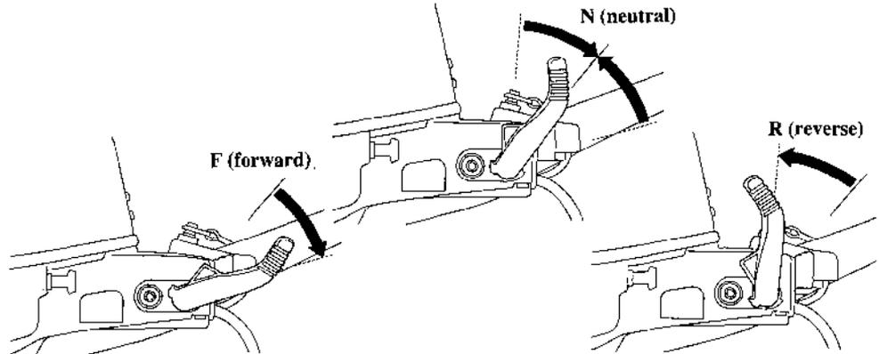
The throttle mechanism is designed to limit the throttle grip travel when operating in the **REVERSE** or **NEUTRAL** positions. The throttle grip can only be turned to the **FAST** position when operating in forward gear.
