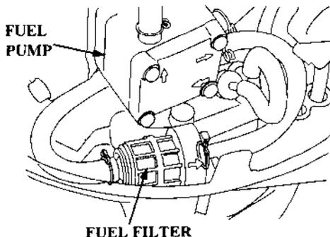
The engine fuel filter is located under the engine cover between the fuel coupling and the fuel pump. Water or sediment accumulated in the fuel filter can cause loss of power or hard starting.
