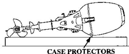
Before removing the motor from the boat, drain the carburetors. Follow the carburetor drain procedure on page 87.
