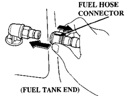
Inspect the fuel hose, and the O-ring seals in the fuel hose connectors. Replace the fuel hose, or fuel hose connectors if they are cracked, damaged or leak fuel. Be sure the fuel hose is not kinked.
