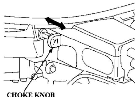
A manual choke knob is provided on the right side of the motor which can be used in the event the battery is discharged. Pull the manual choke knob, and a rich fuel mixture will be provided to the engine.
