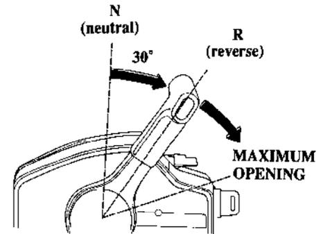
The control lever will not move unless the neutral release lever is pulled up and choke/fast idle lever is in the lowest position.
