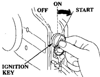
4. Hold the choke/fast idle lever in position, turn the ignition key to the START position and release the key when the engine starts. The starter motor consumes a large amount of current. Do not run it continuously for more than 5 seconds at a time. If the engine does not start within 5 seconds wait at least 10 seconds before using the starter motor again.
