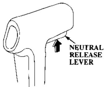
The neutral release lever is on the remote control lever to prevent an accidental gear engagement.
