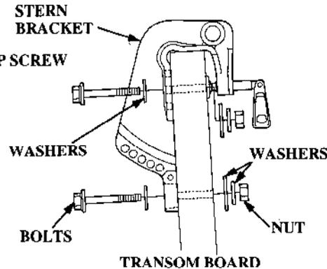
To prevent the outboard motor from falling accidentally, you may further secure the stern bracket to the transom board with the optional Mounting Bolt/ Nut Kit. Good quality stainless steel commercially available bolts, nuts and washers may also be used. Before installing the bolts, be sure to apply sealant to the bolt holes. This modification should be made by your authorized Honda Marine or Honda Outboard Motor dealer. For battery handling and installation information refer to pages 76, 77.
