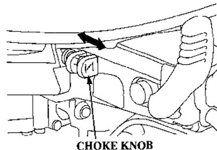
When the engine is cold, pull the choke knob. A rich fuel mixture is provided to the engine by pulling the choke knob.
