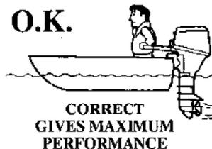
Motor angle controls boat trim. The optimum boat trim is when the boat is parallel with the water. If the boat is not parallel with the water, adjust by changing the position of the transom angle adjusting rod (refer to page 22).
