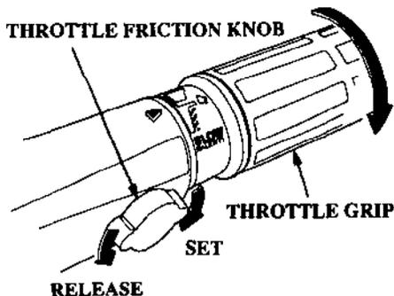
Use the throttle friction knob to set the throttle grip at a certain position while cruising. Turning the friction knob clockwise sets the throttle grip, and it is released by turning the friction knob counterclockwise.
