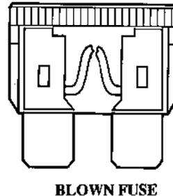
If the fuse is blown, running the engine will not charge the battery and the electric starter will not work.
