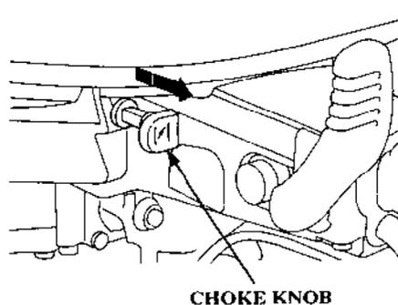
4. When the engine is cold or ambient temperature is low pull the choke knob.
