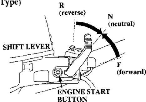
Move the gearshift lever to the N (neutral) position before starting. The engine will not start unless the gearshift lever is in the N (neutral) position.
