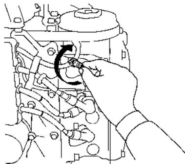
7. Thread the plugs in by hand to prevent cross threading.
