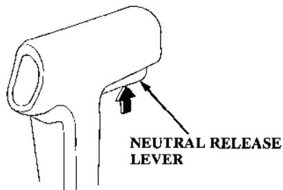
The remote control lever controls gear selection and throttle opening positions.
