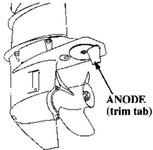
The anode is made from a sacrificial material which helps to protect the outboard motor from corrosion.
