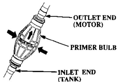
3. Hold the primer bulb so that the outlet end is higher than the inlet end. The arrow on the primer bulb points upward. Squeeze the primer bulb several times until it feels firm, indicating that fuel has reached the carburetors. Check for fuel leaks and repair any leaks before starting the motor.
