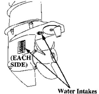
The engine cooling water is drawn into the water pump through these water intakes.
