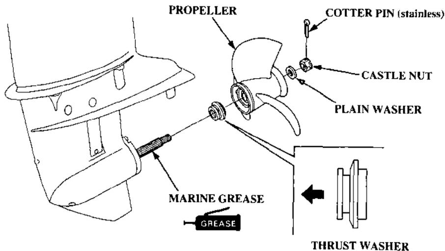
If the propeller is damaged, replace it as follows:
