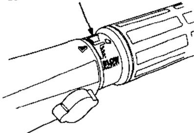
The curve on the grip indicates throttle opening.
