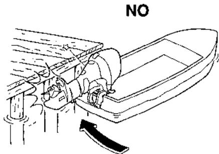
**NOTICE** To avoid damaging the motor, use the utmost care when mooring a boat, especially when its motor is tilted up. Don't allow the motor to strike against the pier or other boats.
