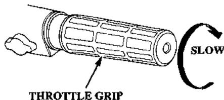
1. Turn the throttle grip to SLOW position and move the gearshift lever to N(neutral).
