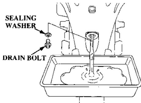
2. Remove the engine oil drain bolt and washer using a 12 mm wrench and drain the engine oil.
