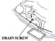
2. With the outboard motor in a vertical position, place an approved gasoline container below the fuel drain outlet, and use a funnel to avoid spilling fuel.
