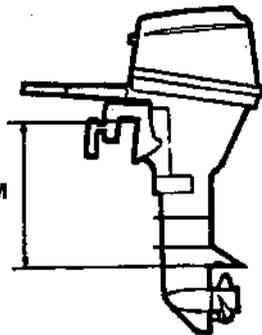
The anti-ventilation plate should be 0–50 mm (0–2 in) below the bottom of the boat. With the boat in the water, loaded and motor off, the anti-ventilation plate should be about 100 mm (3.9 in) below the surface of the water.
