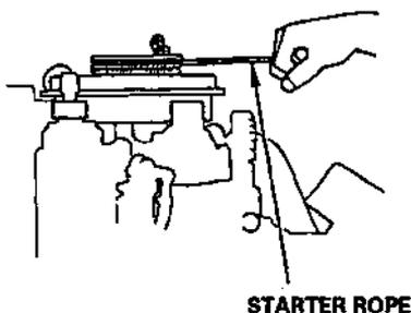
5. Leave the recoil starter off and reinstall engine cover.
