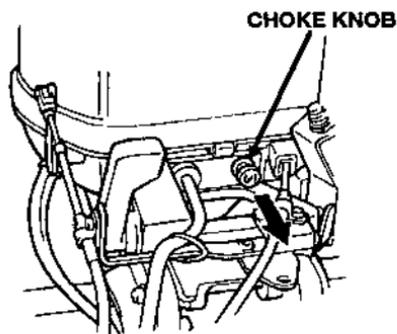
5. Lift the choke/fast idle lever. The choke/fast idle lever will stay up in the fast idle position.
