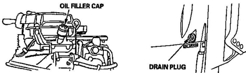
2. Refill to the upper level mark on the oil level dipstick with the recommended oil (see p. 11 ).
