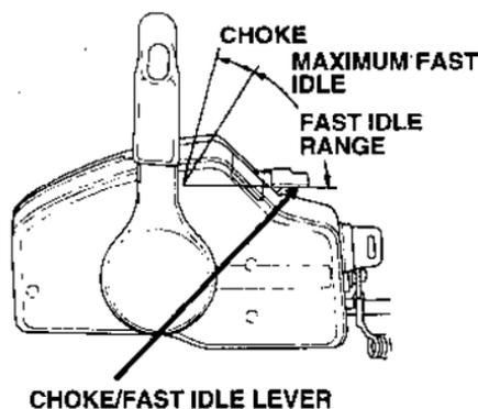
4. While holding the choke/fast idle lever in the up position, turn the ignition key to the START position and release the key when the engine starts. The starter motor consumes a large amount of current. Do not run it continuously for more than 5 seconds at a time. If the engine does not start within 5 seconds wait at least 10 seconds before using the starter motor again.
