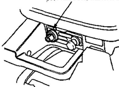
8. After starting, be sure water is flowing out of the water check hole.
