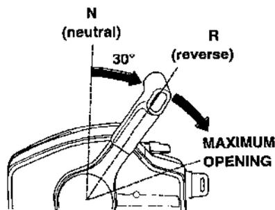
The control lever will not move unless the neutral release lever is pulled up and the choke/fast idle lever is in the lowest position.
