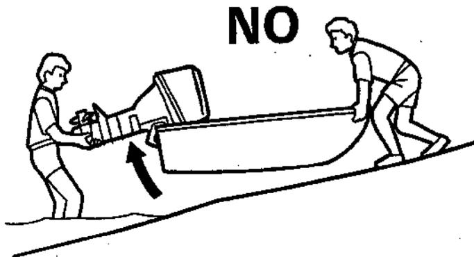
4. Transport and store the motor either vertically or horizontally, as shown below, with the tiller handle raised.
