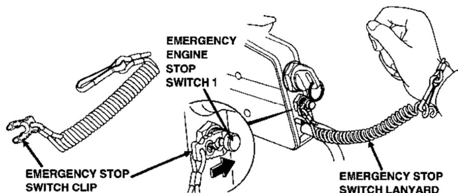
A spare emergency stop switch clip is provided on the remote control box.
