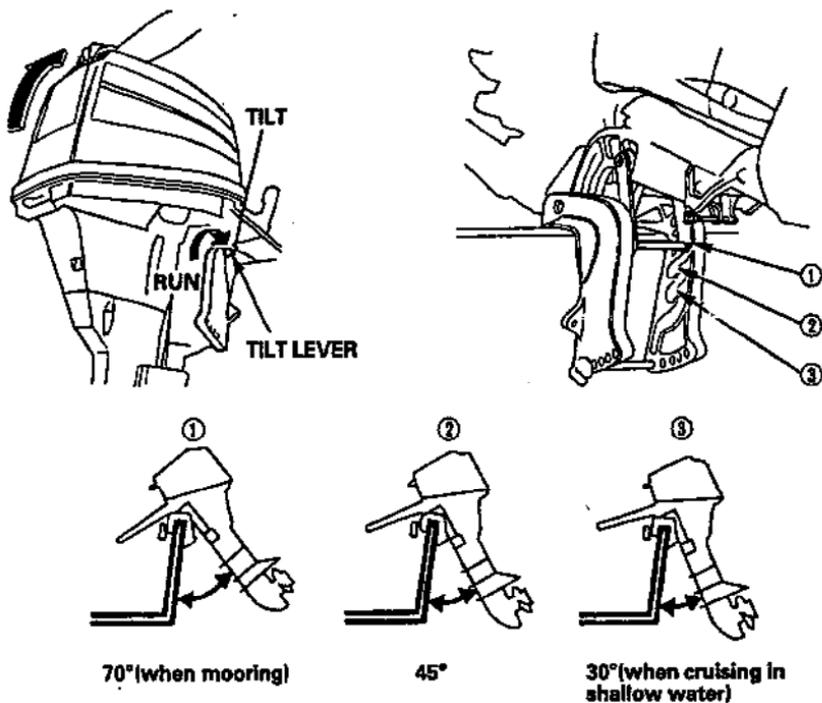
3. To return the engine to the normal RUN position, move the tilt lever away from you until it stops, tilt the engine up slightly, then lower the engine slowly.
