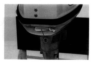
Insert the oil dipstick ① and check the oil level with the dipstick resting on the edge of the filler hole. If the oil level is below the lower level, ③ fill to the upper level.
