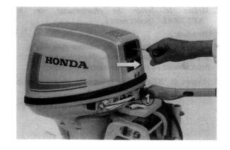
Be sure to check if the oil pressure warning lamp lights. If not, stop the engine immediately, and check the engine oil level and inspect engine for oil leakage.
