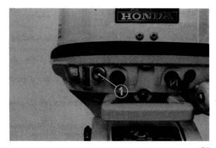
6. After starting, check that water is flowing out of the water check pipe ①.
