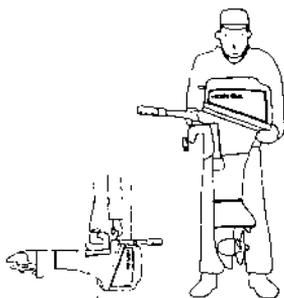
4. Transport and store the motor either vertically or horizontally, as shown here, with the steering handle raised.
