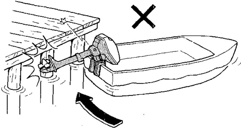
**CAUTION:** To avoid damaging the motor, never use it as a handle for lifting or moving the boat.
