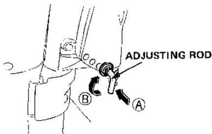
**CAUTION:** To prevent damage to the motor or boat, make sure the adjusting rod is locked.
