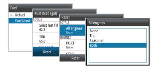
$\rightarrow$  **Note:** You can reset the total for one engine or all engines.
