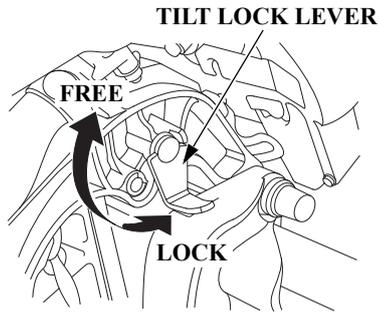
The tilt lock lever is used to support the outboard motor in the fully-raised position.
