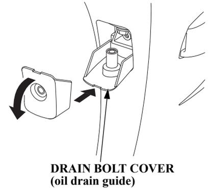
3. Place the drain bolt cover as shown to use it as an oil drain guide. Place a suitable container under the guide.
