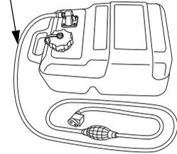
Empty the portable fuel tank into an approved gasoline container. Use a funnel to avoid spilling fuel. Rinse the fuel tank with nonflammable solvent to remove any accumulated sediment.
