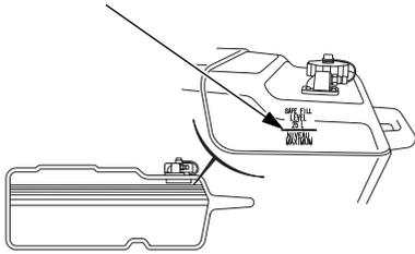
Refuel in a well-ventilated area. Fill the tank to the SAFE FILL LEVEL line.
