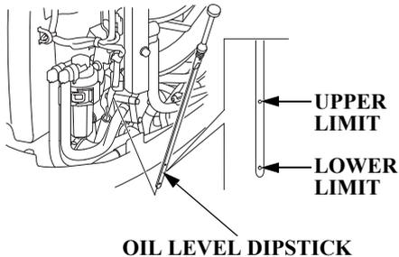
3. Insert the dipstick all the way in, then remove it and check the oil level shown on the dipstick.
