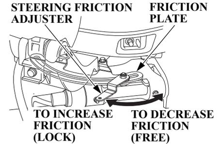
Use the steering friction adjuster to help hold a steady course while cruising.
