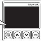
When the alert triggers, the overheat indicator comes on and the buzzer sounds a steady tone as the engine speed is reduced to 1,800 rpm. If the condition persists for another 20 seconds, the engine shuts off. Refer to *TAKING CARE OF UNEXPECTED PROBLEMS*, on p. 130.
