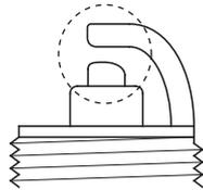
4. Inspect the spark plugs. Replace them if the electrodes are worn, or if the insulators are cracked or chipped.
