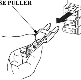
4. Use the fuse puller to remove the fuses. If a fuse is blown, install a replacement fuse of the same specified rating. The outboard motor is supplied with spare fuses in the fuse holder.
