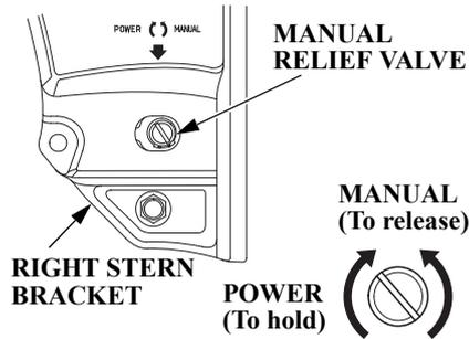
The outboard motor can be tilted manually after opening the manual relief valve. This feature enables the outboard motor to be tilted up or down when no battery is connected.
