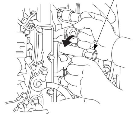
2. Disconnect the spark plug caps from the spark plugs.
