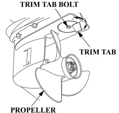
The trim tab compensates for “torque steer,” which is a reaction of the outboard motor to propeller rotation.
