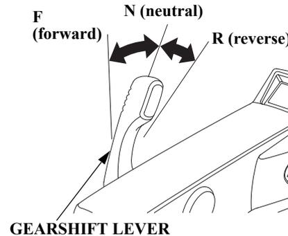
The gearshift lever is used to select F (forward), N (neutral), or R (reverse) gears.
