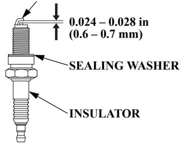
5. Measure the spark plug electrode gap with a wire-type feeler gauge. Correct the gap, if necessary, by carefully bending the side electrode.
