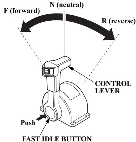
The fast idle button allows you to increase the idle speed without engaging the drive gears. Move the control lever toward the F (forward) or R (reverse) position after pushing in the fast idle button to increase the idle speed.
