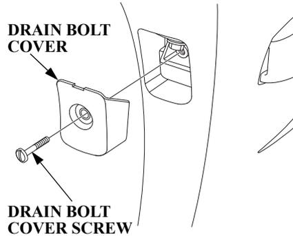
2. Loosen the drain bolt cover screw using a flat blade screwdriver and remove the drain bolt cover.
