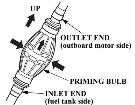
A priming bulb is built into the fuel hose that connects the fuel tank to the outboard motor.
