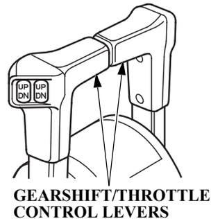
The gearshift/throttle control lever(s) controls engine speed and selects F (forward), N (neutral), or R (reverse) gears.
