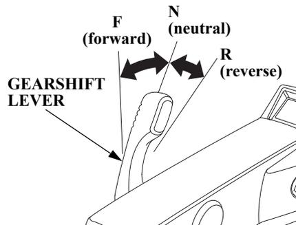
To shift gears, turn the throttle grip to the SLOW position; then move the gearshift lever to select the F (forward), N (neutral), or R (reverse) gears.
