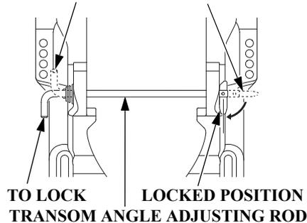
The transom angle adjusting rod limits the tilt angle of the outboard motor when fully lowered.
