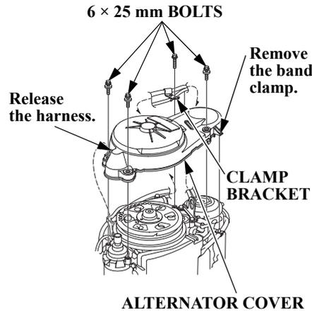
3. Remove the four 6 x 25 mm bolts and clamp bracket, release the harness from the clamber, then remove the alternator cover.
