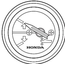
The trim meter indicates the relative trim angle of the outboard motor.
