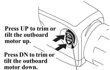
Press UP to trim or tilt the outboard motor up.
