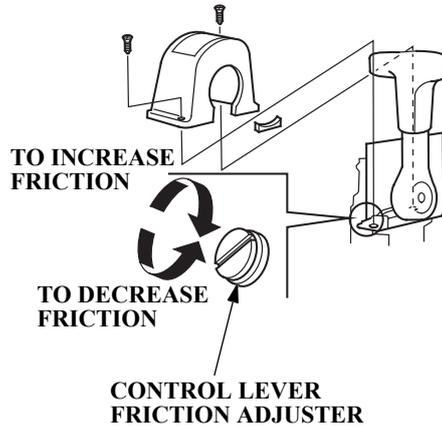
Adjust the control lever friction adjuster so the control lever will hold a constant throttle setting while cruising.
