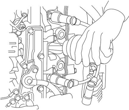
6. Pour 1 – 2 teaspoons (5 – 10 cm<sup>3</sup>) of engine oil into each spark plug hole, and then pull the emergency starter rope several times to lubricate the inside of the cylinders.
