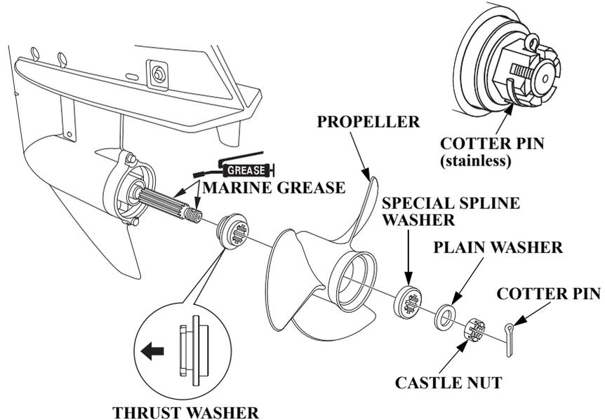
3. Install the propeller, the special spline washer and the plain washer.
