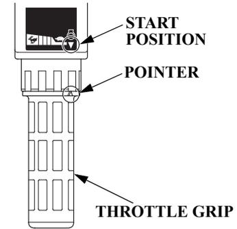
3. Align the engine start symbol "⚙" on the tiller handle with the pointer "▶" on the throttle grip.
