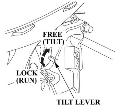
Moving the tilt lever to the FREE (TILT) position allows the outboard motor to be tilted and moving the tilt lever to the LOCK (RUN) position locks the outboard motor in the desired position. Use the tilt lever to temporarily tilt the outboard motor when the boat is operating in shallow water, or mooring in shallow water. The tilt lever must be in the LOCK (RUN) position before operating the outboard motor or the outboard motor could tilt up when operating in reverse.
