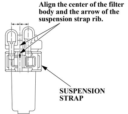
9. Install the suspension strap to the fuel filter assembly as shown above.
