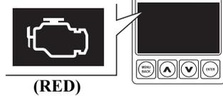
When the engine control system detects an engine control system malfunction, the malfunction indicator turns on and the buzzer sounds at one-second intervals.
