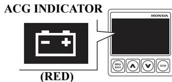
The ACG indicator turns on and the buzzer sounds in one-second intervals when the charging system is faulty.
