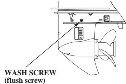
1. Remove the wash screw and sealing washer from the WASH screw hole in the gear case. Be sure not to remove the oil level screw from the OIL LEVEL screw hole in the gear case.
