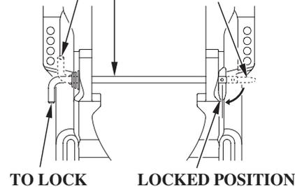
The transom angle adjusting rod limits the tilt angle of the outboard motor when fully lowered.
