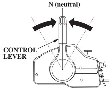
1. Move the throttle grip to the slowest speed and the gearshift lever or control lever to the N (neutral) position.
