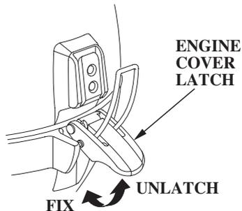
The engine cover latches fasten the engine cover to the outboard motor.
