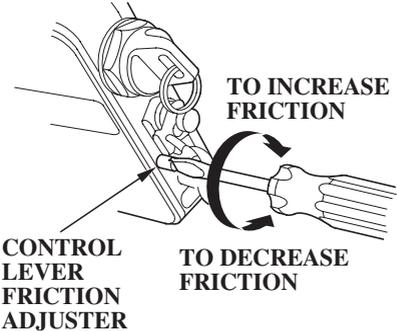
Adjust the control lever friction adjuster so the control lever will hold a constant throttle setting while cruising.
