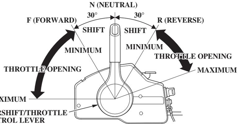
Moving the control lever 30° from N (neutral) selects the gear, and further movement increases engine speed.
