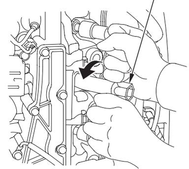
2. Disconnect the spark plug caps from the spark plugs.
