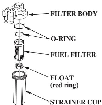
6. Unscrew the strainer cup from the filter body.
