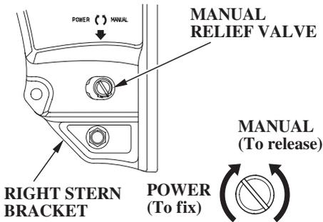
The outboard motor can be tilted manually after opening the manual relief valve. This feature enables the outboard motor to be tilted up or down when no battery is connected.
