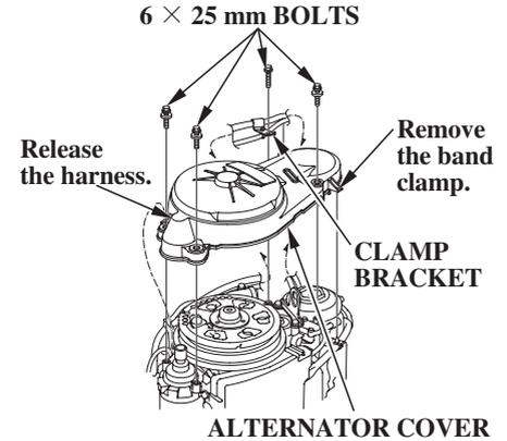
3. Remove the four 6 × 25 mm bolts and clamp bracket, release the harness from the clamer, then remove the alternator cover.
