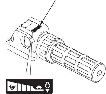
The throttle grip controls engine speed.
