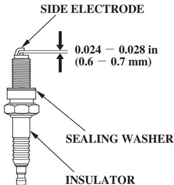
4. Inspect the spark plugs. Replace them if the electrodes are worn, or if the insulators are cracked or chipped.
