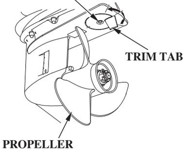
Adjust the trim tab with the engine stopped. Loosen the trim tab bolt above the trim tab, turn the trim tab, and then tighten the bolt securely.
