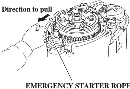
7. Pull the emergency starter rope slowly until resistance is felt, then pull briskly.
