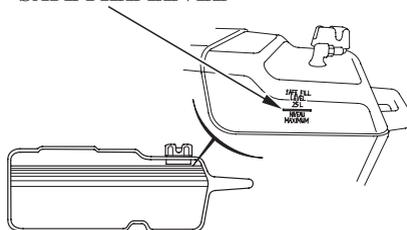
Refuel in a well-ventilated area. Fill the tank to the SAFE FILL LEVEL line.
