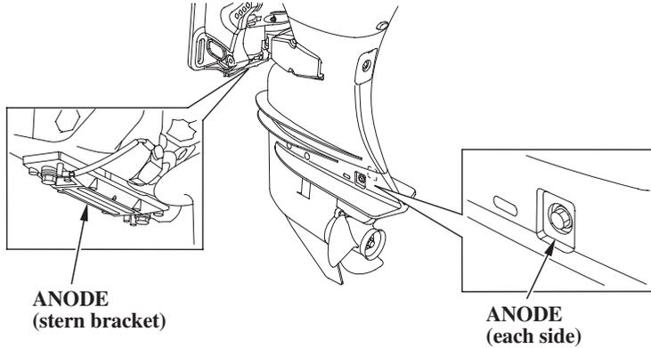
The anodes are made of a sacrificial material that helps to protect the outboard motor from corrosion.
