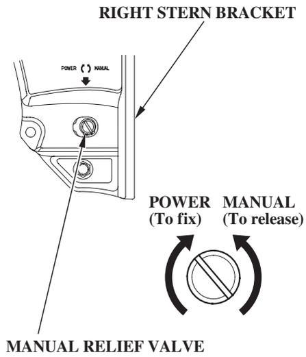
The outboard motor can be tilted manually after opening the manual relief valve. This allows the outboard motor to be tilted up or down when no battery is connected.
