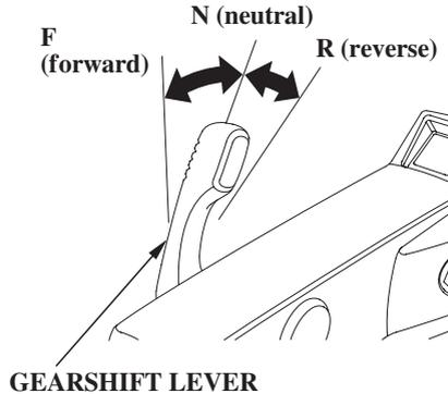
The gearshift lever is used to select F (forward), N (neutral), or R (reverse) gears.
