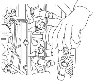
6. Pour 1 – 2 teaspoons (5 – 10 cm<sup>3</sup>) of engine oil into each spark plug hole, then pull the emergency starter rope several times to lubricate the inside of the cylinders.
