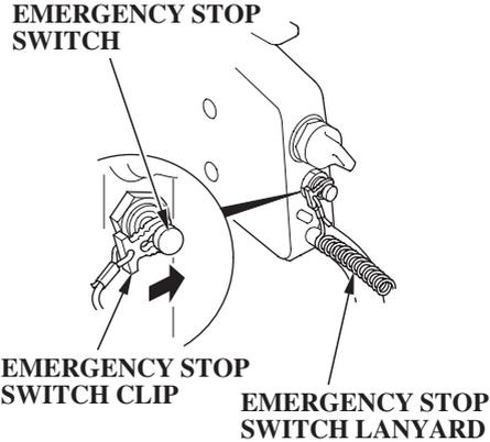
1. Put the emergency stop switch clip in the emergency stop switch, and secure it to the operator or to the operator's PFD (Personal Flotation Device).
