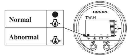
If oil pressure becomes low, the oil pressure indicator will go off, and the engine protection system limits engine speed. If you are at cruising speed, engine speed will decrease automatically.
