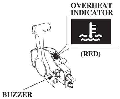
When the alert triggers, the overheat indicator comes on and the buzzer sounds a steady tone as the engine speed is reduced to 1,800 rpm. If the condition persists for another 20 seconds, the engine shuts off. Refer to *TAKING CARE OF UNEXPECTED PROBLEMS*, on p. 106 .
