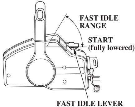
3. Leave the fast idle lever in the START (fully lowered) position.
