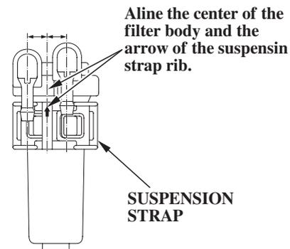
9. Install the suspension strap to the fuel filter assembly as shown above.
