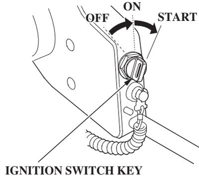
4. Turn the ignition switch key to the ON position; the buzzer will sound twice.
