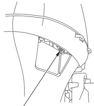
6. Start the engine. Monitor the cooling system indicator. Stop the engine if water does not come out of the cooling system indicator and check the fresh water supply.
