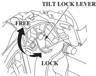
The tilt lock lever is used to support the outboard motor in the fully-raised position.
