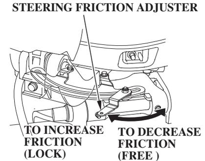
The steering friction adjuster adjusts steering resistance.
