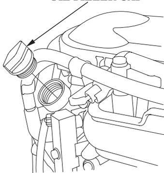
4. If the oil level is low, remove the oil filler cap, and add oil to reach the upper limit mark shown on the dipstick. Use the oil recommended on p. 77.
