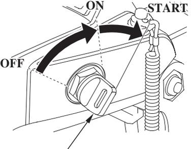
4. Turn the ignition switch key to the ON position; the buzzer will sound twice.
