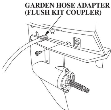
2. Remove the sealing washer from the wash screw and install the sealing washer on the flush kit coupler.
