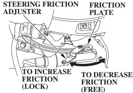
Use the steering friction adjuster to help hold a steady course while cruising.
