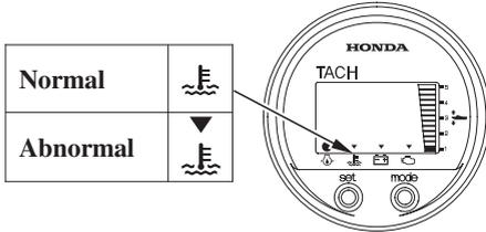
If the engine overheats, the overheat indicator will come on, and the engine will stop in 20 seconds after the engine protection system limits engine speed. If you are at cruising speed, engine speed will decrease automatically.
