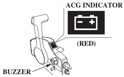
The ACG indicator turns on and the buzzer sounds in one-second intervals when the charging system is faulty.
