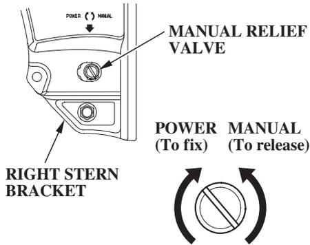
The outboard motor can also be tilted manually after opening the manual relief valve. This feature enables the outboard motor to be tilted up or down when no battery is connected.
