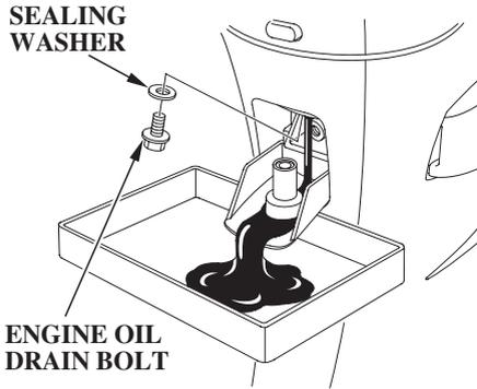
4. Remove the engine oil drain bolt and sealing washer.
