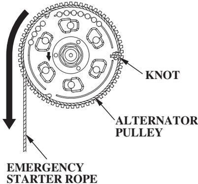
6. Set the alternator pulley so the cutouts are on the right and left sides of the alternator pulley as shown. Hook the knot at the end of the starter rope (accessory) against a cutout in the alternator pulley, and wind the starter rope one and half turns counterclockwise along the groove in the alternator pulley.
