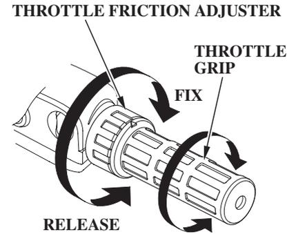
Use the throttle friction adjuster to help hold a constant throttle setting while cruising.
