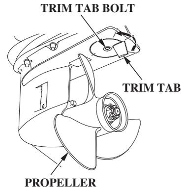
The trim tab compensates for “torque steer,” which is a reaction of the outboard motor to propeller rotation.
