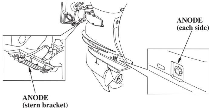
The anodes are located on each side of the gear case and on the stern bracket. They are made of a sacrificial material that helps to protect the outboard motor from corrosion.
