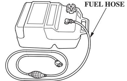
Empty the portable fuel tank into an approved gasoline container. Use a funnel to avoid spilling fuel. Rinse the fuel tank with nonflammable solvent to remove any accumulated sediment.
