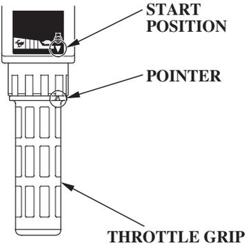
3. Align the engine start symbol “
