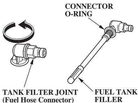
1. Unscrew the fuel hose connector by turning it counterclockwise; then remove the fuel hose connector and fuel tank filter from the tank.
