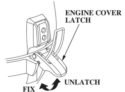
The engine cover latches fasten the engine cover to the outboard motor.
