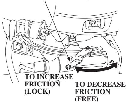
Tighten the steering friction adjuster to prevent the outboard motor from moving while trailering the boat.
