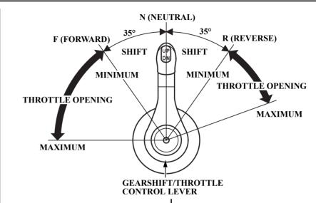
Moving the control lever 35° from N (neutral) selects the gear, and further movement increases engine speed.
