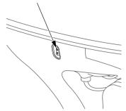
The power tilt switch is located on the engine pan. It is a rocker switch with UP and DN (down) positions for changing the angle of the outboard motor
