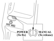
The outboard motor can be tilted manually after opening the manual relief valve. This allows the outboard motor to be tilted up or down when no battery is connected.
