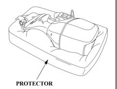
If it is necessary to store the outboard motor horizontally, drain the vapor separator (p. 88 - 89), and drain the engine oil (p. 67), before removing the outboard motor from the boat.
