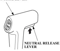
The gearshift/throttle control lever controls engine speed and selects F (forward), N (neutral), or R (reverse) gears.
