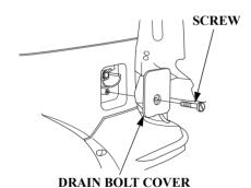
2. Remove the screw from the drain bolt cover, and remove the cover.
