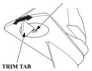
Adjust the trim tab with the engine stopped. Loosen the bolt above the trim tab, turn the trim tab, and then tighten the bolt securely.
