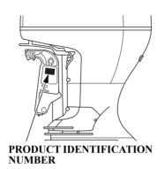
The product identification number is stamped on a plate attached on the left side of the stern bracket
