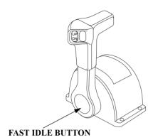
Use the fast idle button to accelerate engine warm-up after starting the engine. Do not use the fast idle button when starting the engine.
