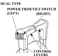
The power trim/tilt switch is located on the control lever. It is a rocker switch with UP and DN (down) positions for changing the angle of the outboard motor
