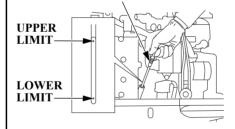
3. Insert the dipstick all the way in, then remove it and check the oil level shown on the dipstick.
