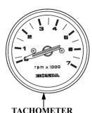
The tachometer shows engine speed in revolutions per minute.
