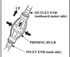
A priming bulb is built into the fuel hose that connects the fuel tank to the outboard motor.
