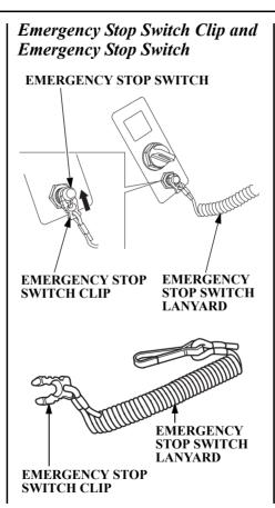
The emergency stop switch clip must be inserted in the emergency stop switch in order for the engine to start and run. The emergency stop switch lanyard must be attached securely to the operator or to the operator's PFD (Personal Flotation Device).
