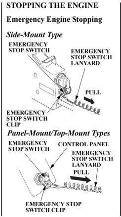
To stop the engine in an emergency, pull the emergency stop switch clip out of the emergency stop switch by pulling the emergency stop switch lanyard.
