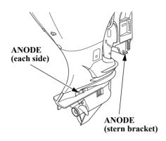
The anodes are made of a sacrificial material that helps to protect the outboard motor from corrosion.
