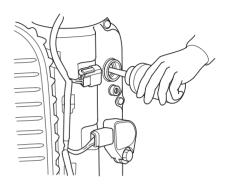
5. Put a teaspoon of engine oil into each spark plug hole to lubricate the inside of the cylinders. Reinstall the spark plugs.
