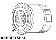
4. Clean the oil filter mounting base, and coat the rubber seal of the new oil filter with clean engine oil.
