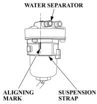
13. Position the aligning mark as shown in the figure when installing the suspension strap on the water separator.
