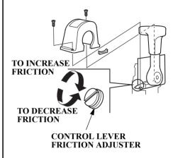
Adjust the control lever friction adjuster so the control lever will hold a constant throttle setting while cruising.
