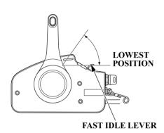
3. Leave the fast idle lever in the OFF (fully lowered) position.
