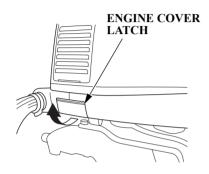
1. Unlock and remove the engine cover (p. 64).
