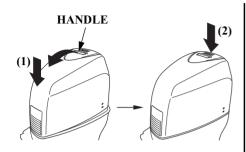
3. While pulling the handle on the engine cover toward you, push the front end of the engine cover down until you hear a click (1), and then push the rear end down until you hear a click (2).
