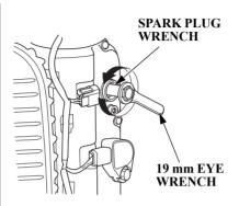
6. Remove the spark plugs with a spark plug wrench and 19 mm eye wrench.
