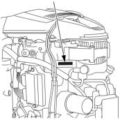
The engine serial number is stamped on the upper right side of the engine.
