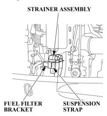
1. Remove the strainer assembly. If it is difficult to remove the strainer assembly by yourself, consult an authorized Honda Marine dealer. Remove the suspension strap from the fuel filter bracket, and then remove the strap from the fuel filter assembly.
