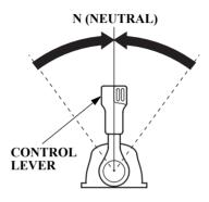
1. Move the control lever(s) to the N (neutral) position.
