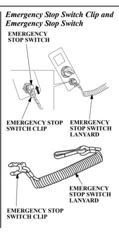
The emergency stop switch clip must be inserted in the emergency stop switch in order for the engine to start and run. The emergency stop switch lanyard must be attached securely to the operator or to the operator's PFD (Personal Flotation Device).
