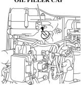
4. If the oil level is low, remove the oil filler cap, and add oil to reach the upper limit mark shown on the dipstick. Use the oil recommended on p. 69.
