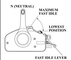
The fast idle lever allows you to increase the idle speed only when the control lever is in the N (neutral) position. Place the fast idle lever in its lowest position to cancel the fast idle and return the control lever to normal operation.
