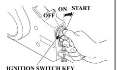
4. Turn the ignition switch key to the ON position; the buzzer will sound
