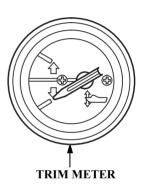
The trim meter indicates the relative trim angle of the outboard motor.
