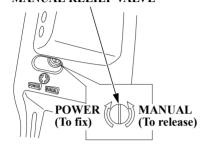
The outboard motor can be tilted manually after opening the manual relief valve. This feature enables the outboard motor to be tilted up or down when no battery is connected.
