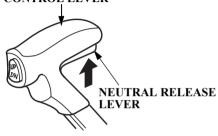
The gearshift/throttle control lever controls engine speed and selects F (forward), N (neutral), or R (reverse) gears.
