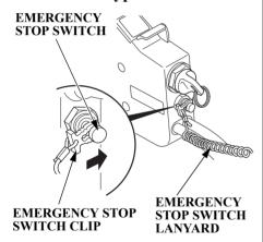
1. Put the emergency stop switch clip in the emergency stop switch, and attach the emergency stop switch lanyard securely to the operator or to the operator's PFD (Personal Flotation Device).
