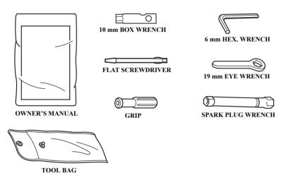
The tool kit can be used for simple maintenance procedures and emergency repairs. Keep these items on the boat so that they will always be available if you need them.
