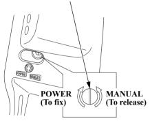
The outboard motor can also be tilted manually after opening the manual relief valve. This feature enables the outboard motor to be tilted up or down when no battery is connected.
