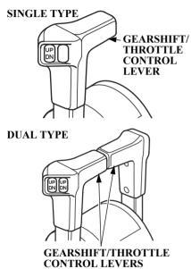
The gearshift/throttle control lever(s) controls engine speed and selects F (forward), N (neutral), or R (reverse) gears.
