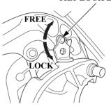
The tilt lock lever is used to support the outboard motor in the fully-raised position.
