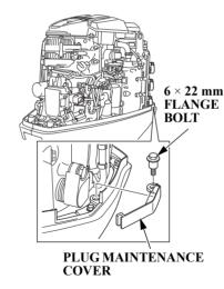
3. Remove the 6 × 22 mm flange bolt and remove the plug maintenance cover.
