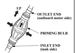
Hold the priming bulb up in the direction of the arrow; then squeeze the priming bulb several times until it feels firm, indicating that fuel has reached the engine.
