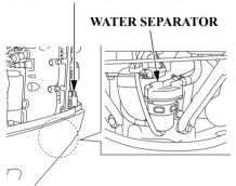
The water separator is located under No. 6 cylinder ignition coil. Water accumulation in the water separator can cause loss of power or hard starting. Check the water separator periodically. Clean it or consult with an authorized Honda Marine dealer for cleaning.
