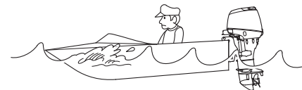
INCORRECT CAUSES BOAT TO "BOW STEER"
