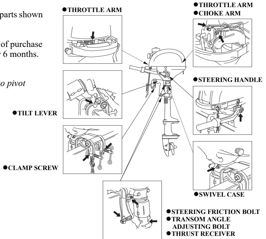
Apply Honda Marine Corrosion Inhibitor (or equivalent) to all areas under the engine cover and any exposed metal surfaces.
