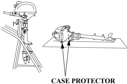
If storing horizontally, be sure to fold the tiller handle, and rest the outboard motor on its case protectors.
