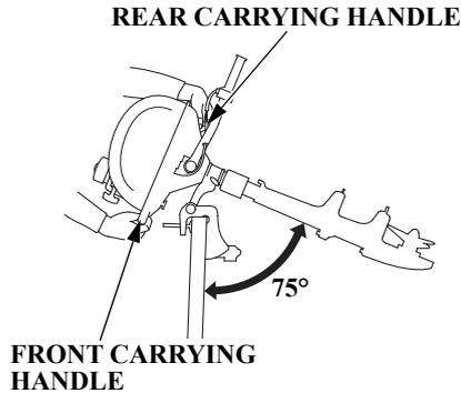
The tilt lever enables the outboard motor to be tilted for beaching, launching, or mooring.
