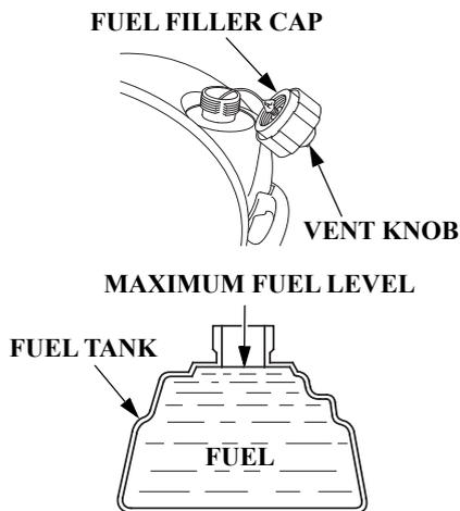
Refuel in a well-ventilated area. Fill the tank to the maximum fuel level.
