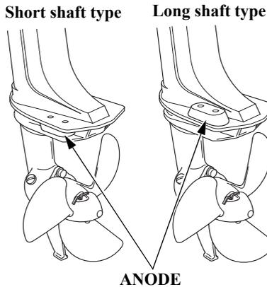
The anode is made of a sacrificial material that helps to protect the outboard motor from corrosion.
