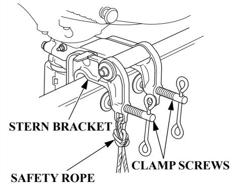
Attach the stern bracket to the boat transom by tightening the clamp screws.
