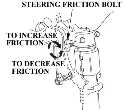
The steering friction bolt adjusts steering resistance.
