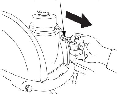
Inspect the recoil starter rope, and replace it if it becomes frayed.
