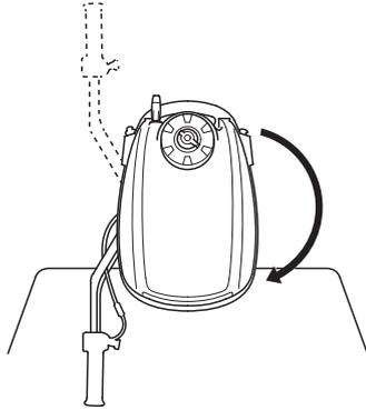
2. To reverse direction, turn the outboard motor 180°, and then pivot the tiller handle as shown. Be careful not to hold and move the throttle grip when pivoting the tiller handle.
