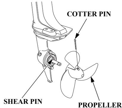
Remove the cotter pin, then remove the propeller and shear pin.
