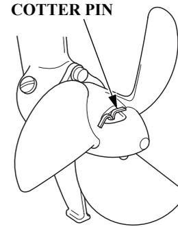
Install the propeller in the reverse order of removal. Be sure to replace the cotter pin with a new one.
