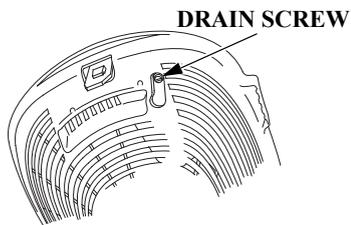
4. After draining is completed, tighten the carburetor drain screw and turn the fuel valve lever to the OFF position.
