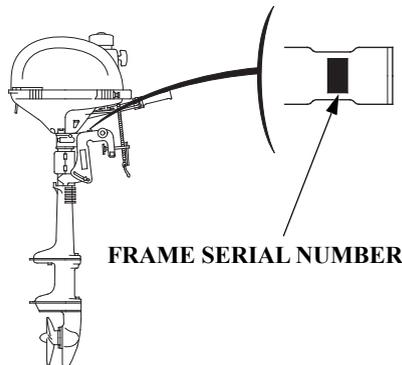
The frame serial number is stamped on a plate attached on the upper part of the swivel case.
