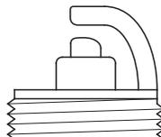
4. Inspect the spark plug. Replace it if the electrode is worn, or if the insulator is cracked or chipped.
