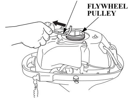
4. Set the knotted end of the emergency starter rope in the notch in the flywheel pulley. Wind the rope clockwise around the flywheel pulley, as shown.
