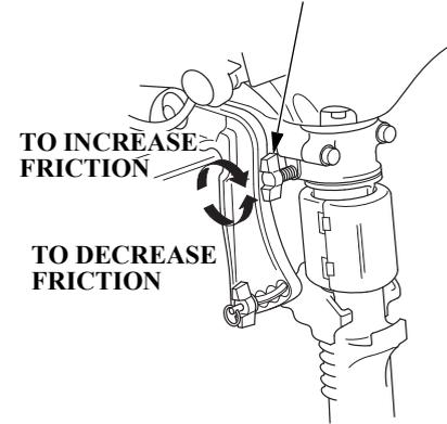
Use the steering friction bolt to help hold a steady course while cruising.
