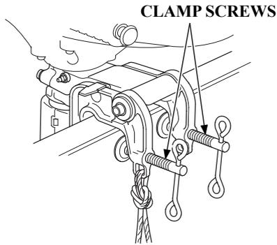
Use the clamp screws to secure the outboard motor to the transom.
