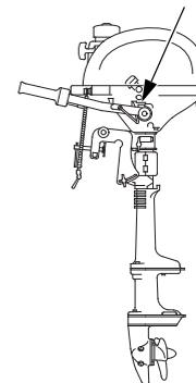
The engine serial number is stamped on a plate attached on the clutch housing.
