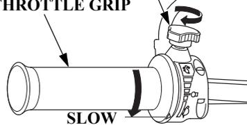
1. Move the throttle grip to the SLOW position and hold it there by turning the throttle grip friction knob clockwise.
