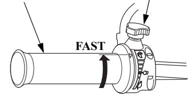
Use the throttle grip friction knob to help hold a constant throttle setting while cruising.
