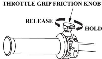
The throttle grip friction knob adjusts resistance to throttle grip rotation.
