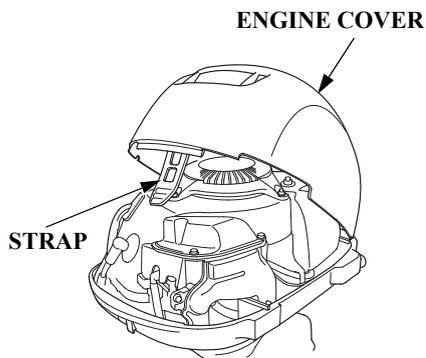
The engine cover retaining strap fastens the engine cover to the outboard motor.
