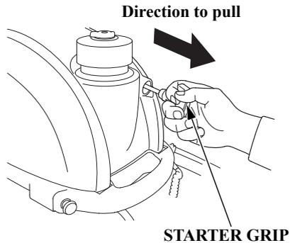
Pulling the starter grip operates the recoil starter to crank the engine for starting.
