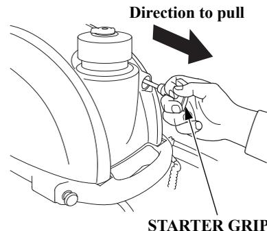
4. Remove the spark plug (p. 48), and remove the emergency stop switch clip from the emergency stop switch. Pull the starter grip, rotate the flywheel a few revolutions to completely expel any water from the cylinder.
