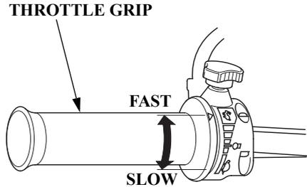
The throttle grip controls engine speed.
