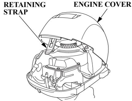
Use the retaining strap to hold the engine cover closed. Do not remove the engine cover while the engine is running.
