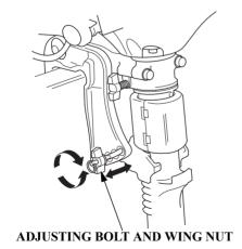
The transom angle adjusting bolt is used to adjust the angle of the outboard motor in the normal operating position (p. 34).
