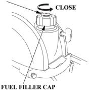
4. Close the fuel tank vent by turning the vent knob to the OFF position.
