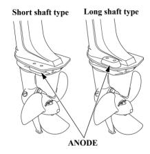
The anode is made of a sacrificial material that helps to protect the outboard motor from corrosion.
