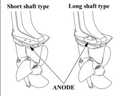
The anode is made of a sacrificial material that helps to protect the outboard motor from corrosion.
