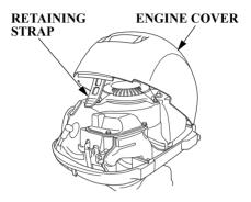
Use the retaining strap to hold the engine cover closed. Do not remove the engine cover while the engine is running.
