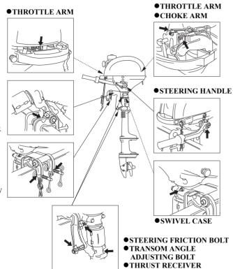
Apply Honda Marine Corrosion Inhibitor (or equivalent) to all areas under the engine cover and any exposed metal surfaces.
