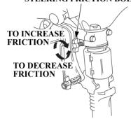
The steering friction bolt adjusts steering resistance.
