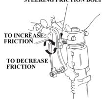
Use the steering friction bolt to help hold a steady course while cruising.
