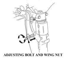
The transom angle adjusting bolt is used to adjust the angle of the outboard motor in the normal operating position (see page 34).
