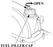
2. Open the fuel tank vent by turning the vent knob to the ON position.
