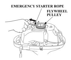
4 Set the knotted end of the emergency starter rope in the notch in the flywheel pulley. Wind the rope clockwise around the flywheel pulley, as shown.
