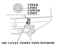
1. Check the oil level shown on the oil level inspection window.
