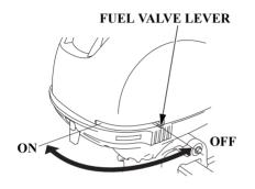
The fuel valve opens and closes the passage between the fuel tank and the carburetor.
