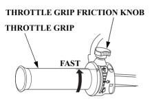
Use the throttle grip friction knob to help hold a constant throttle setting while cruising.
