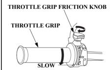
1. Move the throttle grip to the SLOW position and hold it there by turning the throttle grip friction knob clockwise.
