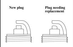
4. Inspect the spark plug. Replace it if the electrode is worn, or if the insulator is cracked or chipped.
