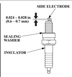
5. Measure the spark plug electrode gap with a wire-type feeler gauge. Correct the gap, if necessary, by carefully bending the side electrode
