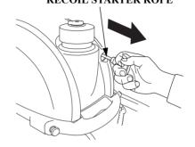
Inspect the recoil starter rope, and replace it if it becomes frayed.
