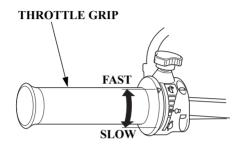
The throttle grip controls engine speed.
