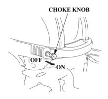
5. To start a cold engine, pull the choke knob to the ON position. To restart a warm engine, leave the choke knob in the OFF position.
