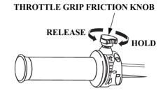
The throttle grip friction knob adjusts resistance to throttle grip rotation.
