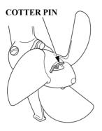
Install the propeller in the reverse order of removal.
