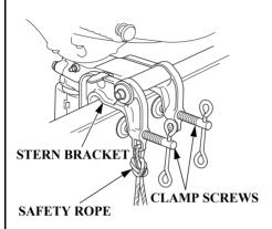
Attach the stern bracket to the boat transom by tightening the clamp screws.
