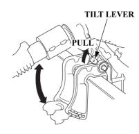
5. To return the outboard motor to the normal running position, hold the outboard motor by the front carrying handle on the engine case and pull the tilt level toward you, and then lower the outboard motor slowly.
