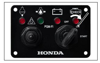
4. Press the emergency stop switch button five times within 20 seconds. The buzzer will sound once indicating the hour counter has been reset.
