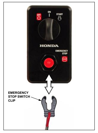
5. Return the shift lever(s) to the neutral position, and then turn the ignition switch(es) OFF.
