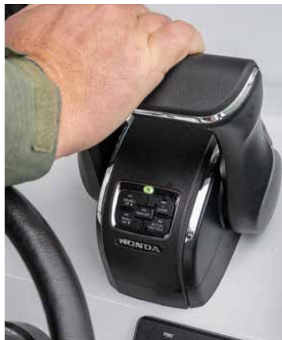
Honda's iST® drive-by-wire controller with 5-button interface combines ergonomics and comfort with superior functionality for confident boating.
