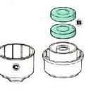
\* Wash "B" and "C" in cleaning solvent, after drying, refill with clean engine oil up to oil level mark.
