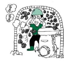
WARNING: \* Exhaust contains poisonous carbon monoxide gas.
