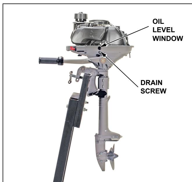
7. Reinstall the oil drain screw and a new washer.
