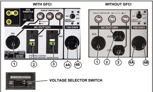
When the voltage selector switch is in the 120V/240V position, receptacle 4 supplies up to 22.9A at 240 volts from the combination of power circuits A and B.
