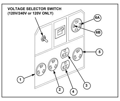
When the voltage selector switch is in the 120V only position, terminal 6A supplies up to 30 amps at 120 volts from power circuits A and B; terminal 6B has no power.
