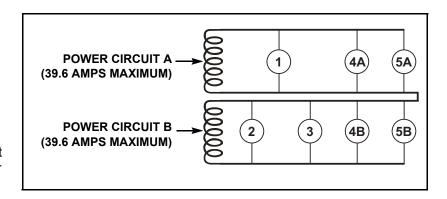
If you need 240 volt power, receptacle 4 (the combination of 4A and 4B) can provide up to 30 amps at 240 volts (the receptacle is only rated at 30 amps). Receptacle 5 (5A and 5B) can provide up to 39.6 amps at 240 volts (the receptacle is rated at 50 amps).
