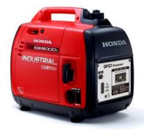
Similar to the EU2000*i*, the new EB2000*i* offers inverter power with a maximum output of 2,000 watts with Honda's fuel-efficient Eco-Throttle<sup>™</sup>. The Eco Throttle<sup>™</sup> feature allows the generator to conserve fuel by varying engine rpm to produce only the power required to operate the equipment, improving fuel economy. Additionally, the
