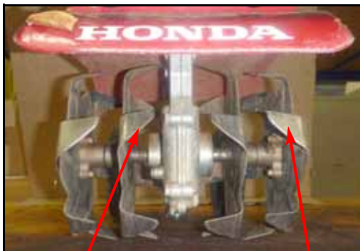
CORRECT INSTALLATION (Viewed from the front)
