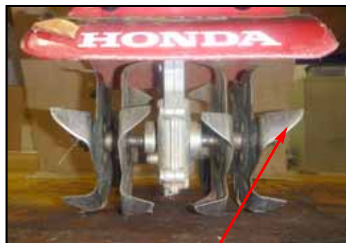
INCORRECT INSTALLATION (Viewed from the front)
