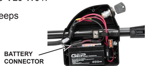
1. Remove the battery cover by removing the three cover mounting screws, and then disconnect the battery connector.
