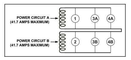
If you use 240 volt power, receptacle 3 (the combination of 3A and 3B) can provide up to 30 amps at 240 volts (the receptacle is only rated at 30 amps). Receptacle 4 (4A and 4B) can provide up to 41.7 amps at 240 volts (the receptacle is rated at 50 amps).
