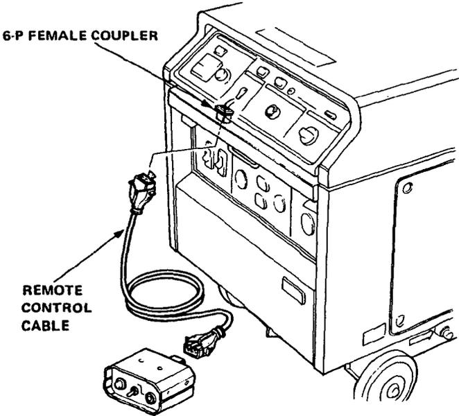
7. Connect the remote control 6-P male coupler to the switch box.
