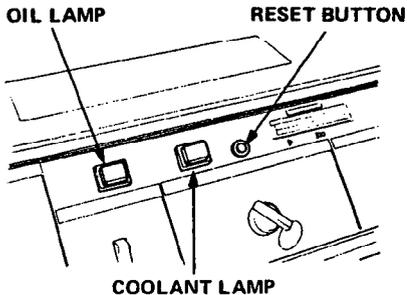
**CAUTION:** If engine idle speed is set too low, the protection circuit cannot be activated while idling. The correct idle speed is  $2200 \pm 200$  rpm.
