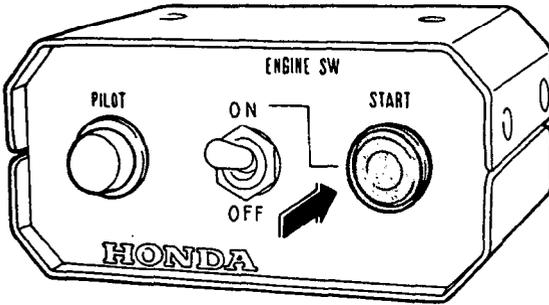
**NOTE:** Do not hold the starter button on for more than 15 seconds at a time.
