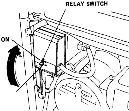
6. Flip the remote control engine switch knob up to ON.
