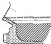
Fill sump with SE rated SAE 10W-40 engine oil: 0.45ℓ
