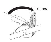
Release the drive clutch lever (SD, S3D).
