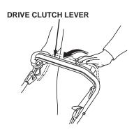
Operate the drive clutch lever with a quick and complete motion, so the drive clutch is either fully engaged or released. Hold the drive clutch lever against the handlebar during self-propelled mowing. This will help to extend the service life of the clutch mechanism.
