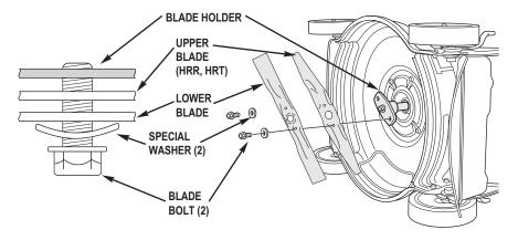
3. **Installation:** Clean around the blade holder. Install the blade(s) using the bolts and special washers as shown (concave side of the special washers toward the blade(s)).
