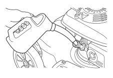
4. Fill with the recommended oil. Do not overfill; measure the oil level as shown on page 34.
