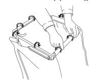
Lift the rear door, remove the mulching plug, then install the grass bag.
