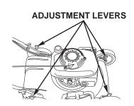
If you are not sure what cutting height to select, start with a high setting and check the appearance of the lawn after mowing a small area. Readjust cutting height if necessary.
