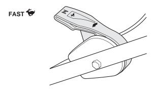
When you need to leave the mower for any reason, move the throttle to SLOW, then turn the engine OFF by releasing the flywheel brake lever.
