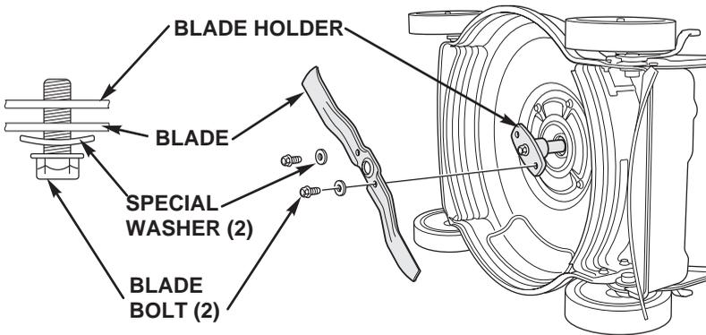
The blade bolts and washers are specially designed; when replacing them, use only genuine Honda parts. Tighten the bolts with a torque wrench. Use a wooden block to stop the blade from turning.
