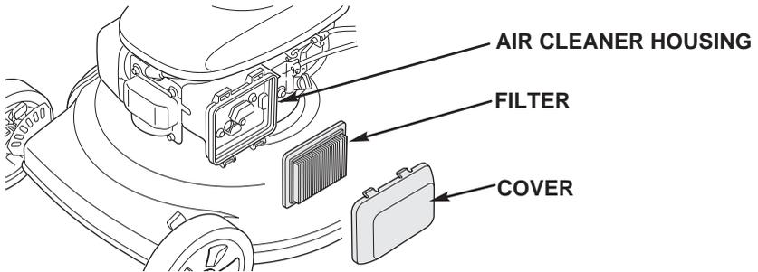
2. Clean the filter by tapping the filter several times on a hard surface to remove dirt, or blowing compressed air (not exceeding 30 psi [207 kPa]) through the filter from the inside. Never try to brush off dirt; brushing will force dirt into the fibers.
