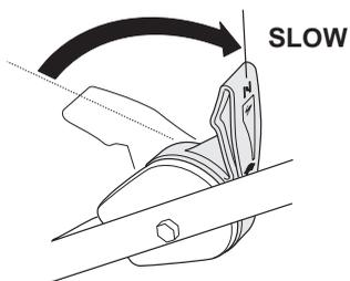
2. Release the drive clutch lever (SD).
