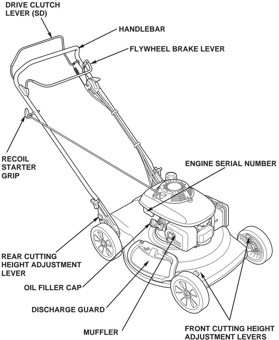
HRS216PD: Manually propelled (push)
