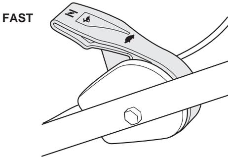
When you need to leave the mower for any reason, always turn the engine OFF by releasing the flywheel brake lever.
