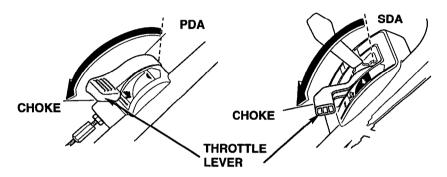
2. The choke arm should move counterclockwise, until it contacts the stop post on the carburetor.
