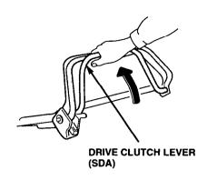
Operate the drive clutch lever with a quick and complete motion, so the drive clutch is either fully engaged or released. Hold the drive clutch lever against the handlebar during self-propelled mowing. This will help to extend the service life of the clutch mechanism.
