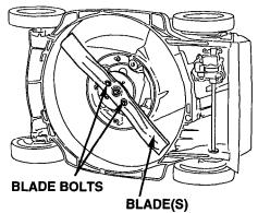
4. Inspect blade(s) for wear and damage.
