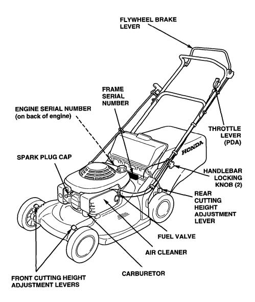
Record the frame and engine serial numbers in the space below. You will need these serial numbers when ordering parts and when making technical or warranty inquiries (see page 84).
