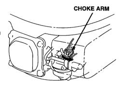
4. If the choke arm does not move all the way to its stop, in either direction, take the mower to an authorized Honda servicing dealer. Throttle cable adjustment involves related control plate adjustments.
