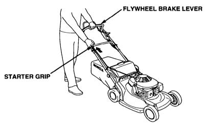
6. If the CHOKE position was used during starting, move the throttle lever away from the CHOKE position as soon as the engine warms up enough to run smoothly. Set the throttle lever at FAST to mow or at SLOW to idle.
