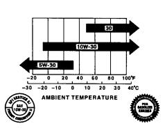
The SAE oil viscosity and service classification are in the API label on the oil container. Honda recommends that you use API SERVICE category SH or SJ oil with the ILSAC "starburst" certification mark displayed on the container.
